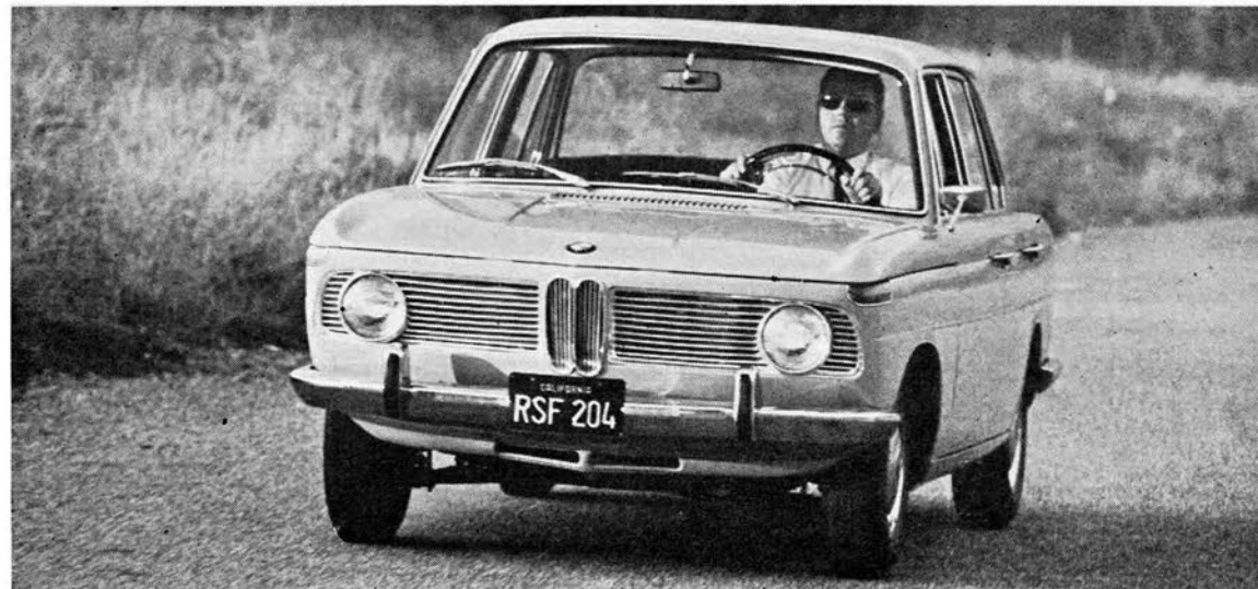
BMW IS NOT NEARLY SO TALL (57½ INCHES) AS THE LOW HOOD, EXPANSIVE GLASS, AND 6.00 X 14 TIRES MAKE IT LOOK.
