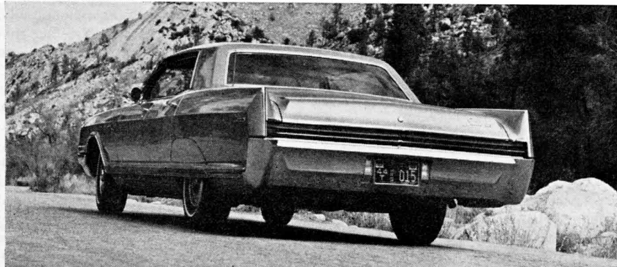
Tail lights stretch entire width of body. Suspension is well isolated from frame, thereby reducing transmission of road noise to a minimum. Brakes proved excellent in mountains.
