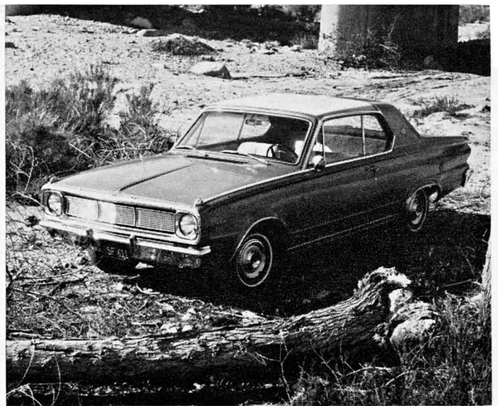
Vinyl top insert of the GT is held by chrome trim which causes a strong, irritating wind noise at moderate to high road speeds.
