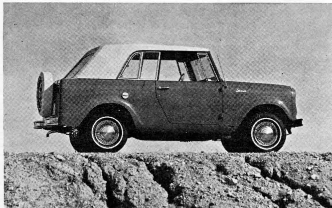
Fiberglass top and rear windows are removable, chromed bumpers are standard on Sportop. Two side-filling tanks are optional.
