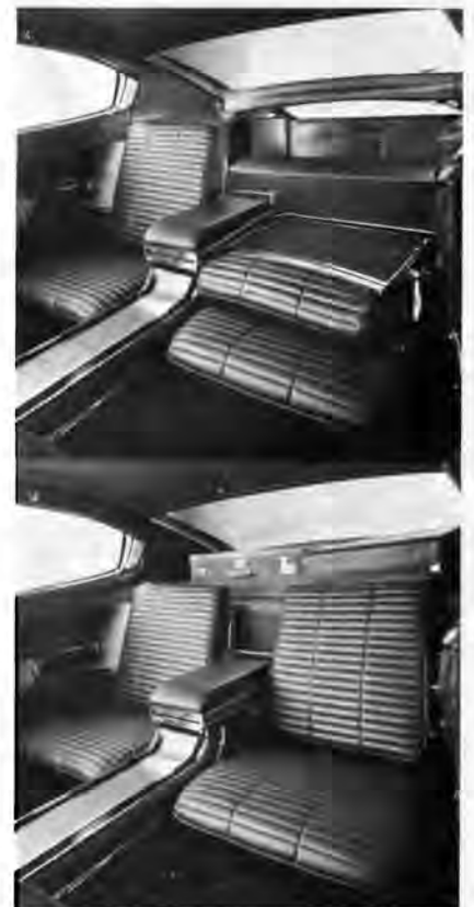
Novel interior has full-length console over driveshaft tunnel, individual seats which fold down for additional luggage space. Interior communicates with trunk.
