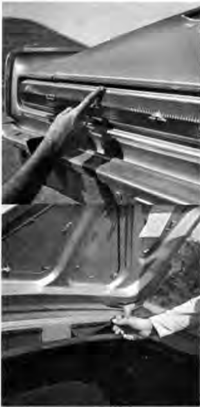
Flow-through fresh air system uses adjustable front vents and slot under deck lid for entry and exit. Rubber flaps cover holes in deck frame.
