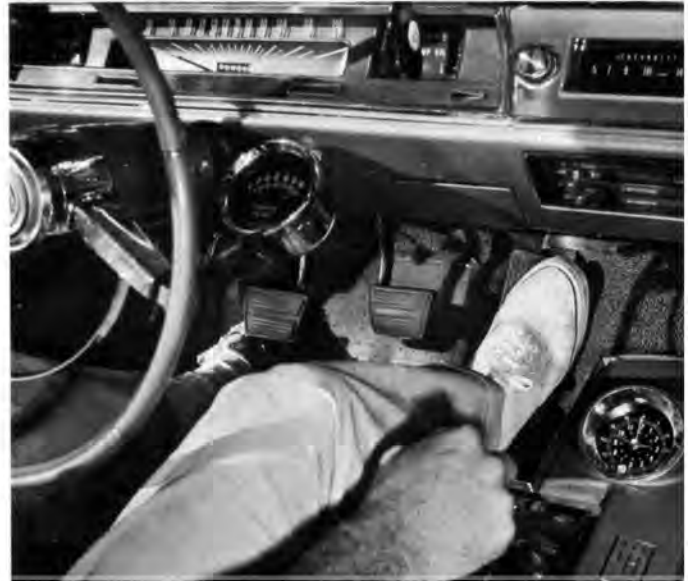
Position of brake and accelerator pedals is not conducive to hard driving. Shift lever action is quick, positive.
