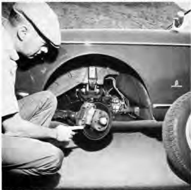
Girling power-assisted disc brakes are fitted to front wheels with drum type at rear. Braking capability is in line with performance.
