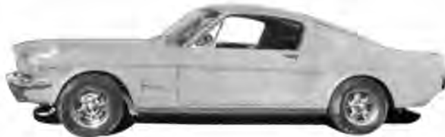
V8 4-Speed, 271 hp (modified). Zero to 60: approximately 8.5 seconds. Fuel economy 15-17 mpg. Price: $3,650 plus.
