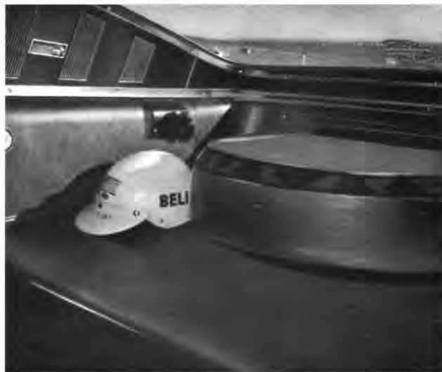
Rear seat space in Shelby 350 is usurped by spare tire moved from luggage compartment to make room for big tank.
