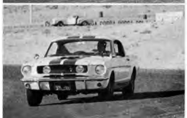
Four Mustangs at same speed in same corner at Willow Springs Raceway exhibit different handling characteristics. Six has more roll but less understeer than 1966 V8. Moontang's wider base wheels make it more neutral. Shelby 350 is loafing through turn where others are working.
