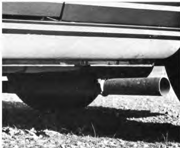
Straight-through mufflers and short exhaust pipes ending in front of rear wheels are part of Shelby package.
