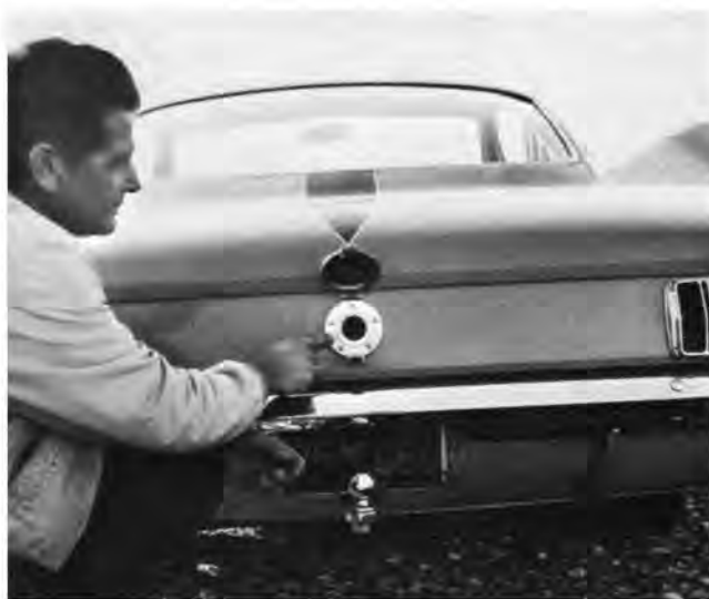
Substitution of Moon quick-fill gas cap for stock Mustang cap ended thefts of this attractive item.
