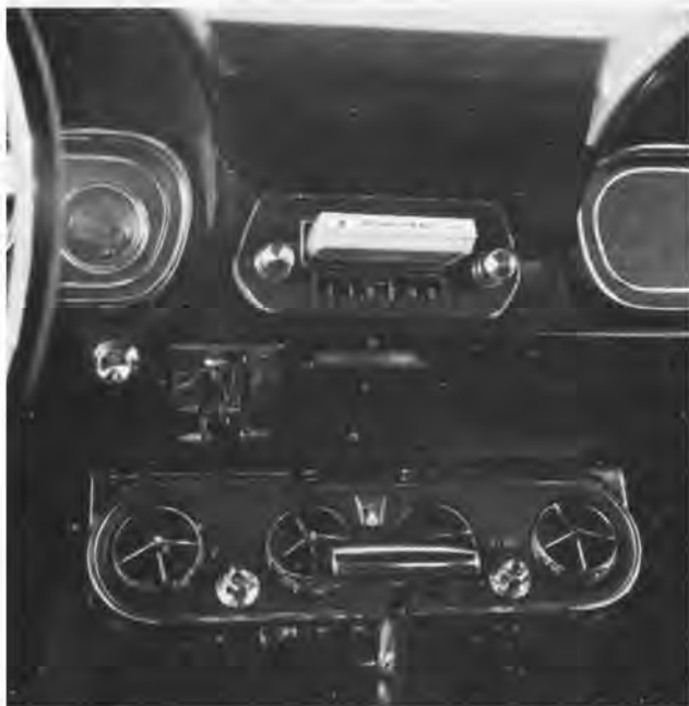
Air conditioning unit and floor-shift for automatic eliminate center of front seat as adult passenger spot.
