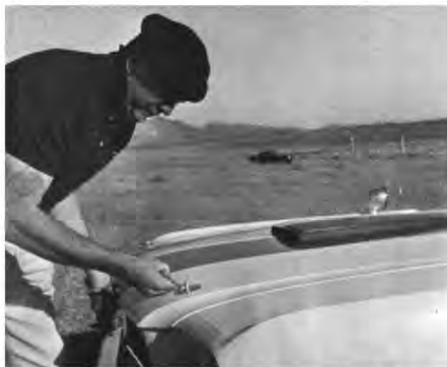
Fiberglass hood on 350 is secured by pin-lock of type used on racing cars. Scoop is functional, stripes cost extra.
