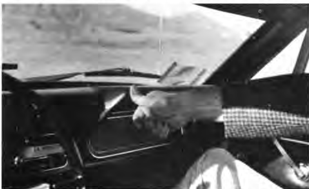
Unyielding, sharp edged padding for top of Mustang dash is poor design feature, offers an unnecessary hazard.
