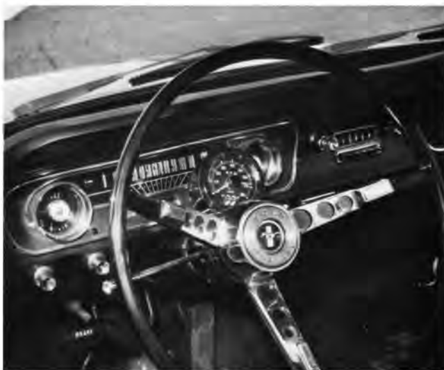
Additions to 1965 HP V8 by owner include Moon tachometer mounted on steering column. Car has been used as rolling test bed for speed equipment.
