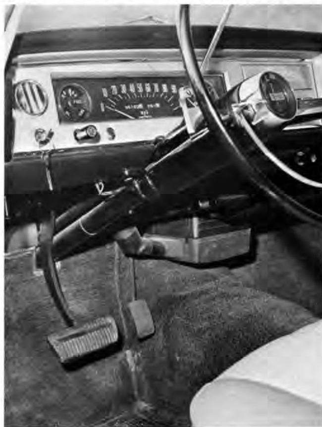
Speedometer is big, legible. Accelerator and brake pedals are near same height. Air vent above ignition key delivers fresh air.
