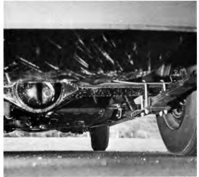
Corona is undercoated by factory at no extra cost. Rear suspension is conventional live-axle type.
