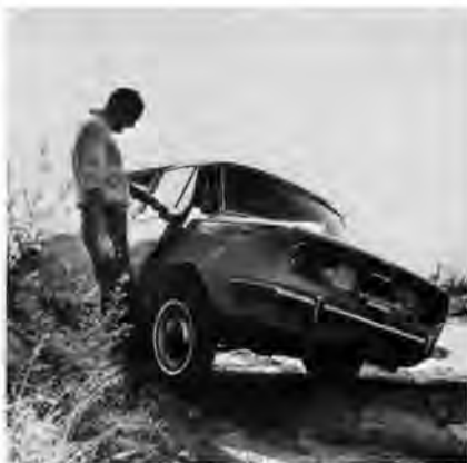
Unit construction body has good torsion rigidity. Doors can be opened under severe twisting.
