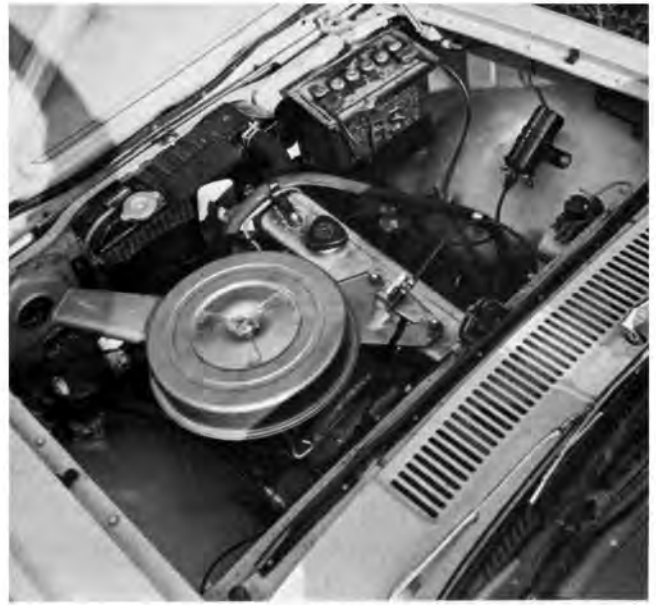
Toyota engine is 116 cubic inch four, develops 90 horsepower, has outstanding low speed torque.
