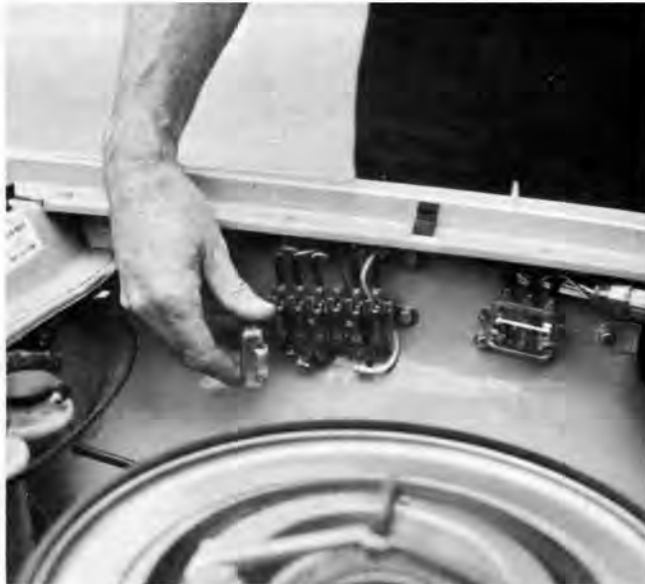
Fuse block is located handily in engine compartment which is neat, orderly and easy to service.
