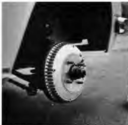
Finned aluminum front brake drums improve fade-resistance. Lining-to-weight ratio is favorable.
