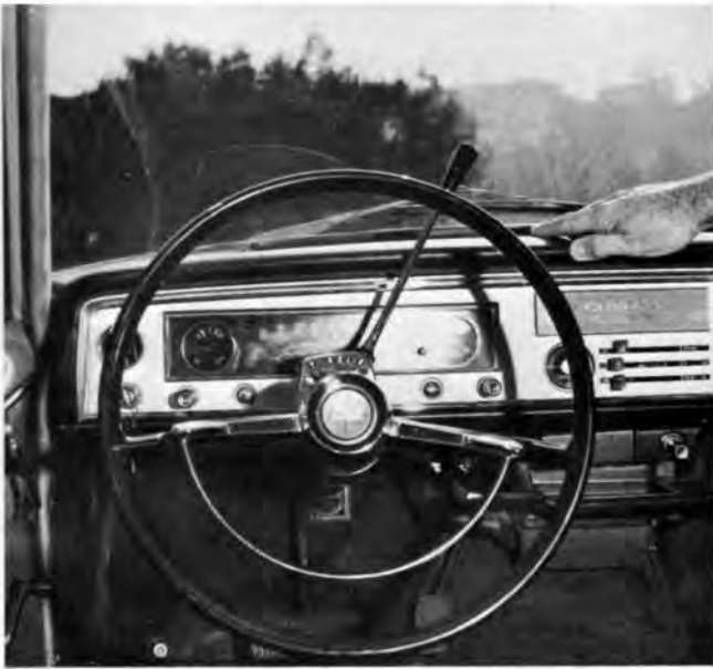
Automatic shift lever is on steering column, has familiar P N D L R arrangement of U.S. autos.
