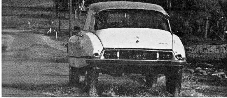
Control in driver's compartment increases road clearance by nearly six inches to facilitate fording streams and crossing rough terrain. When a tire is changed, the car is first raised and then let down on a stand inserted under the desired side.
