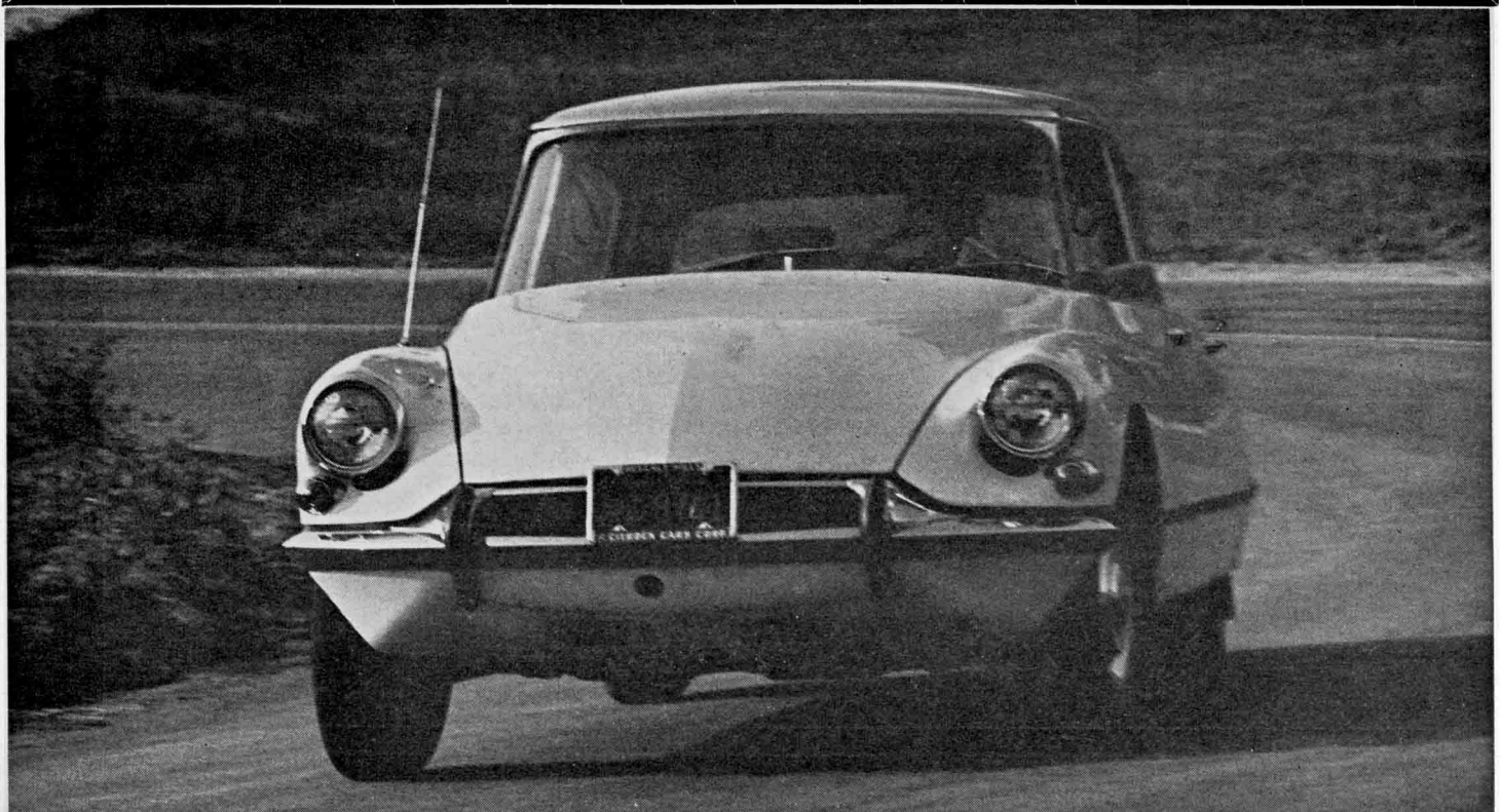
TWO LOWER SCOOPS DIRECT AIR TO INBOARD FRONT DISCS. THE MAIN SCOOP ABOVE DIRECTS AIR THROUGH A CHUTE TO THE RADIATOR.
