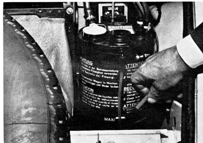
Accumulator for central hydraulic system has visual gauge to check level of automatic transmission fluid used. From this are operated the automatic clutch, suspension units, brakes, power steering, and self-leveling and height-control features.
