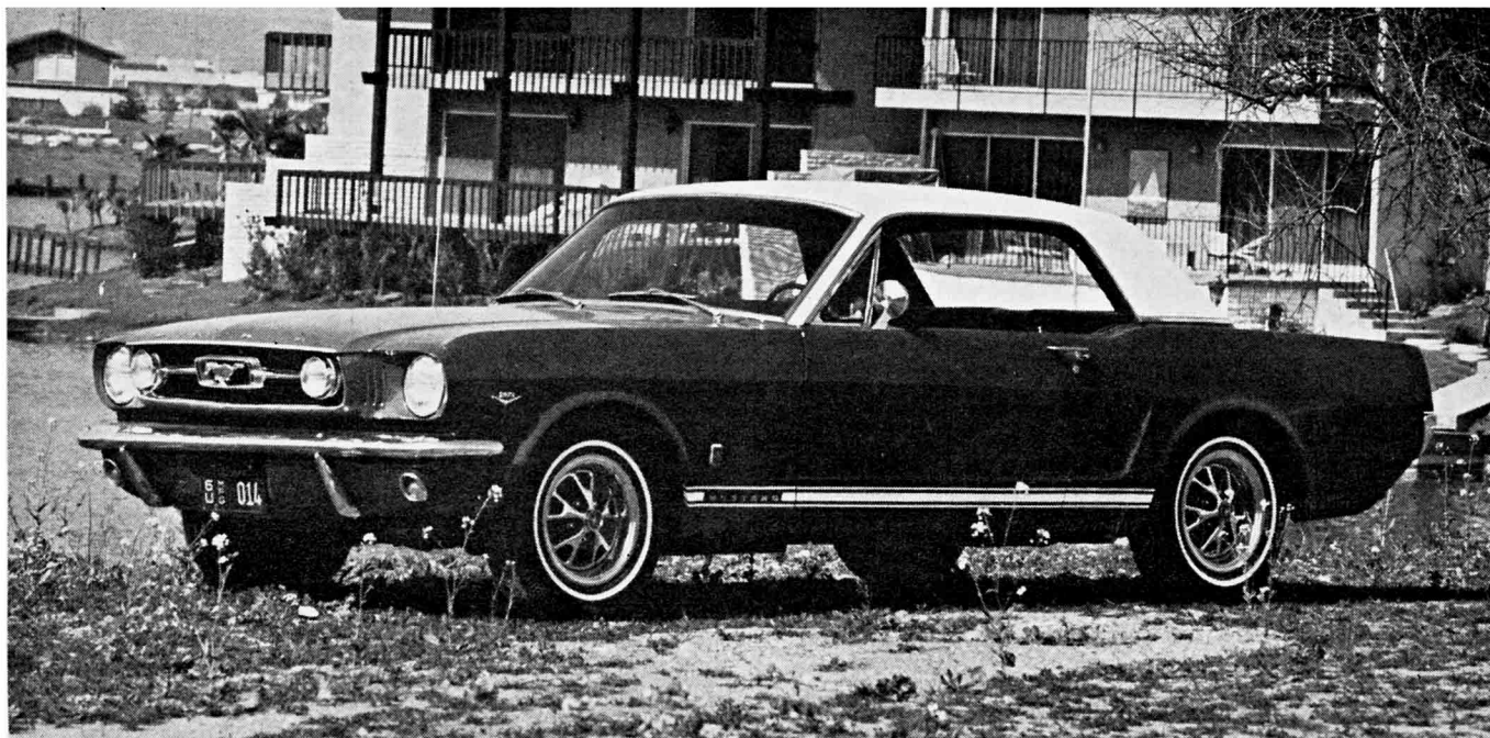
FOG LAMPS AND RACING STRIPE ARE BOTH PART OF OPTIONAL GT KIT. EXTRA-COST WHEELS ADD ATTRACTIVE TOUCH TO CAR'S CLEAN LINES.
