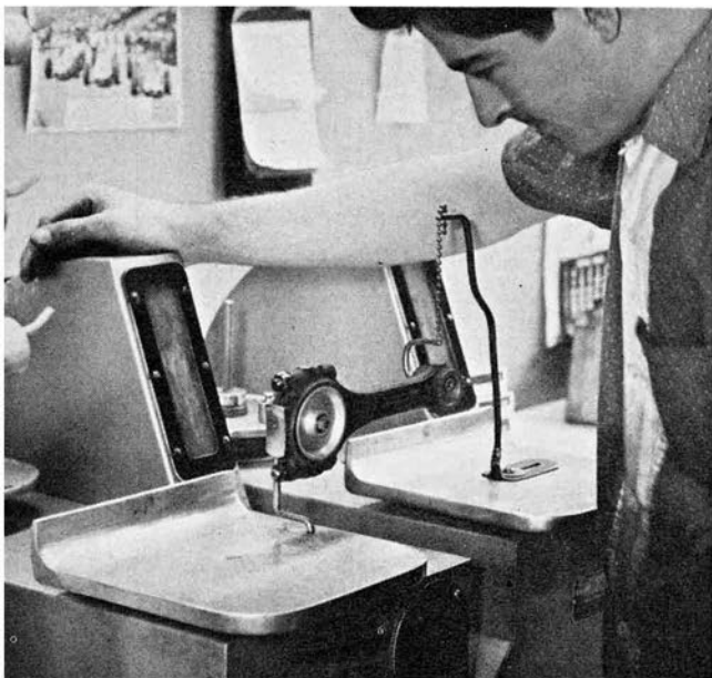
Rods must be inspected and replaced if defective. They must be matched for weight, and small ends balanced to within one gram.
