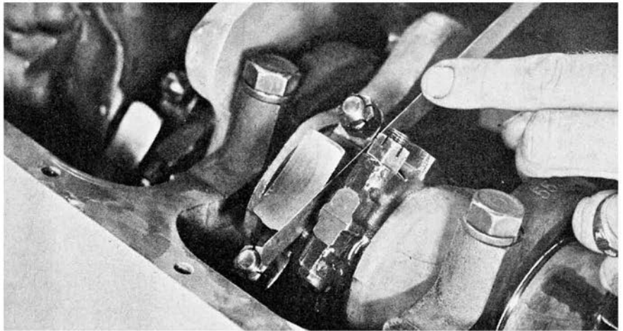
After rods caps are slightly tightened, check the end play between rods and also at main bearing thrust surface. End play for clearance must be adequate when engine is running at higher power settings.
