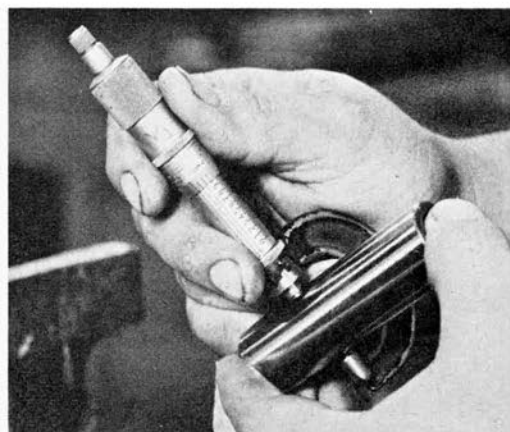
Pins should be miked at both ends and middle to detect any taper; use only quality pins.
