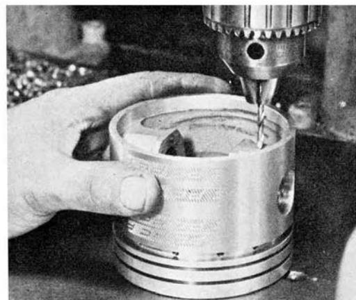
Small holes are drilled in piston pin boss from bottom up to increase the amount of oil at piston/pin area.
