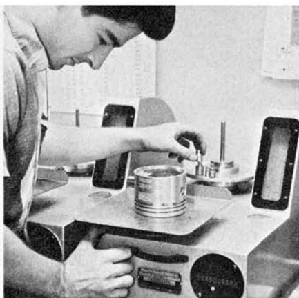
Early ohv engines were not balanced as well as current crop, so matching piston weight is vital.
