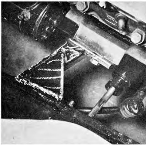
Stock motor mounts were retained, new frame mount towers built from rectangular tubing.
