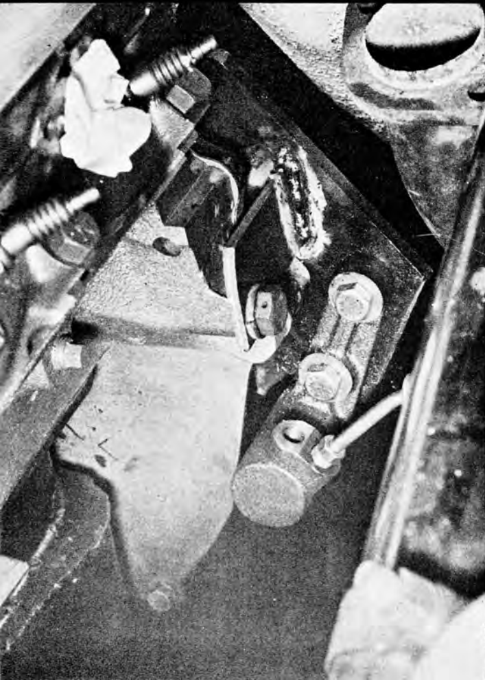
BELOW RIGHT — Hurst floor shift conversion takes up more space than original automatic floor shifter, so large hole was cut in flooring tunnel, later covered with metal patch.
