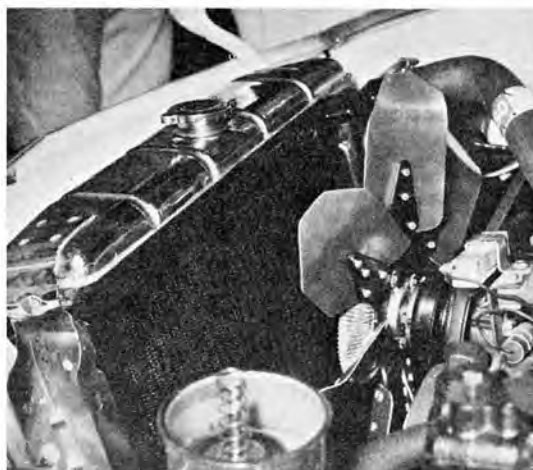
Eaton seven-blade temp-a-trol fan was installed. It fits well behind stock radiator location.
