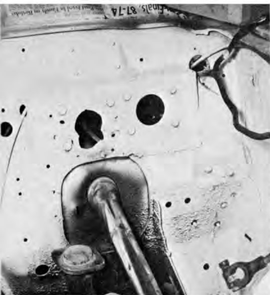
Ford pickup swinging pedal brake and clutch assembly were bolted in.
