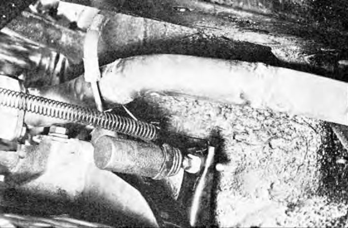
ABOVE — New header pipe from 289 exhaust manifold must be made in S bend.
