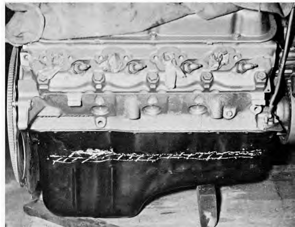
Stock 289 pan has sump in front. This pan was cut in two, one-inch section added for more depth, then sump put in rear to clear crossmember.
