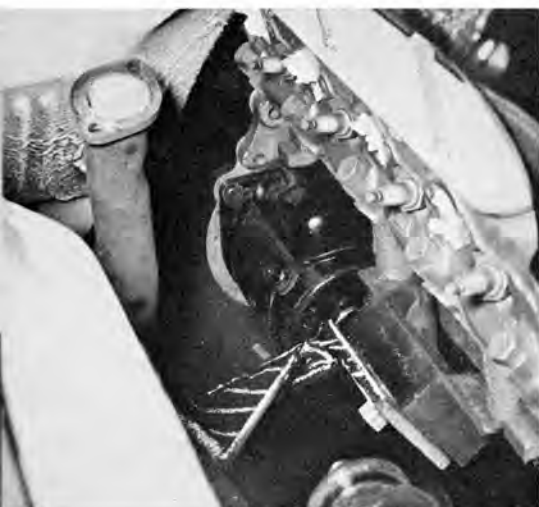
Another view of stock T-Bird header pipe. Pickup slave cylinder operates stock 289 throwout arm.
