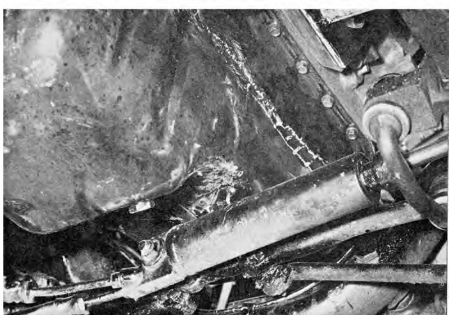
Clearance between reworked oil pan and steering links/crossmember is more than enough (about 2-1/2 inches).
