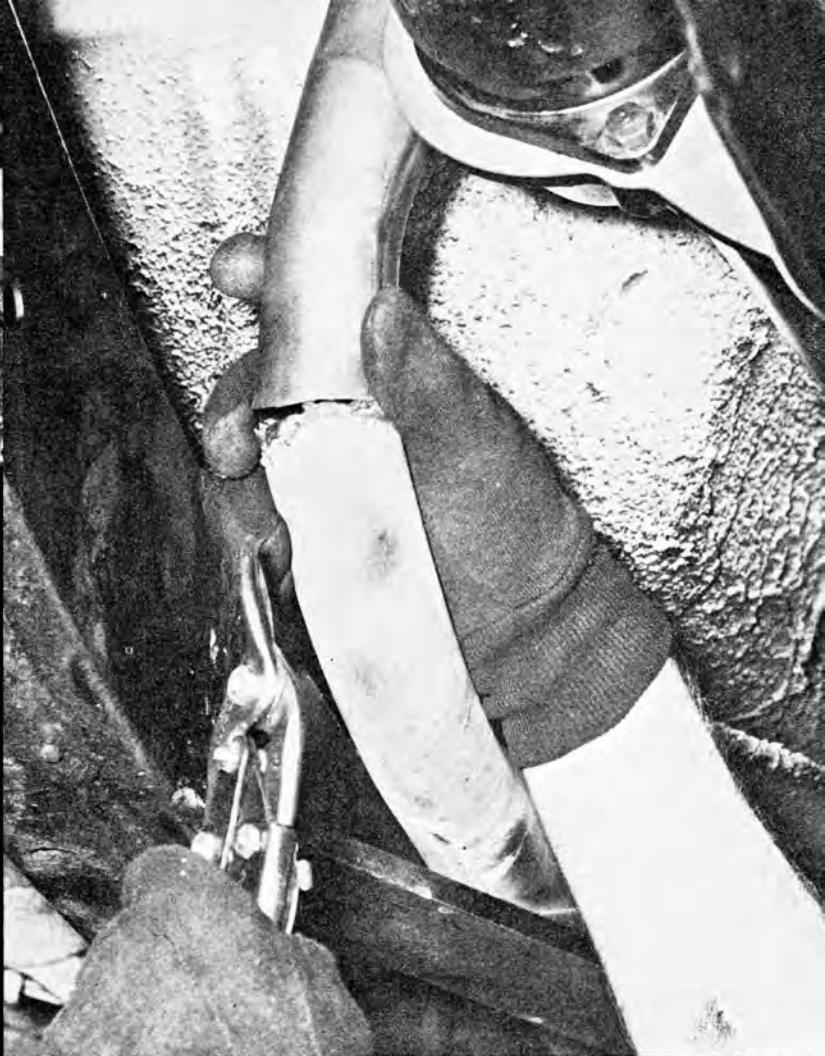
BELOW RIGHT — Hurst floor shift conversion takes up more space than original automatic floor shifter, so large hole was cut in flooring tunnel, later covered with metal patch.
