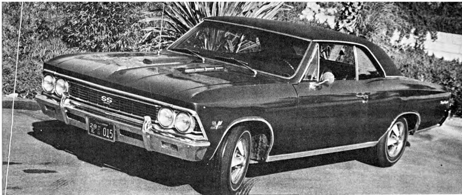
Hood scoops denote the 396-cubic-inch engine. Car weight is well distributed for drag racing performance.
