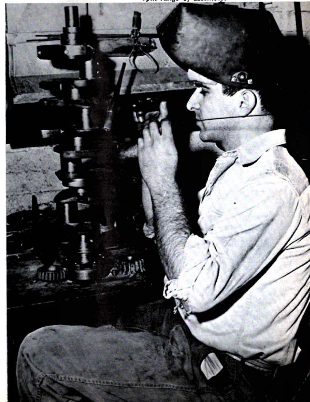
Counterweight is heli-arc welded on each side of the center main to eliminate crank flexing and extend rpm range of assembly.
