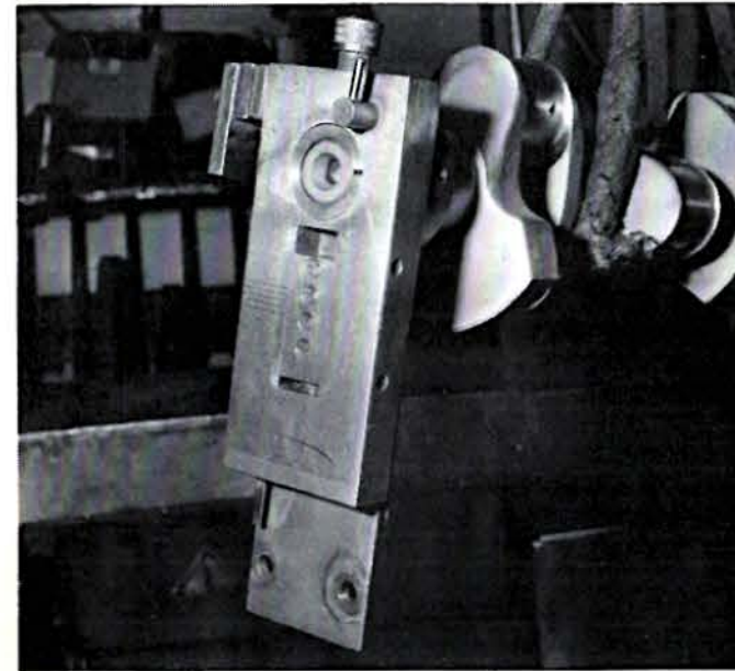
Cranks are positioned on special throw blocks to insure that the throws are ground 90 degrees apart.
