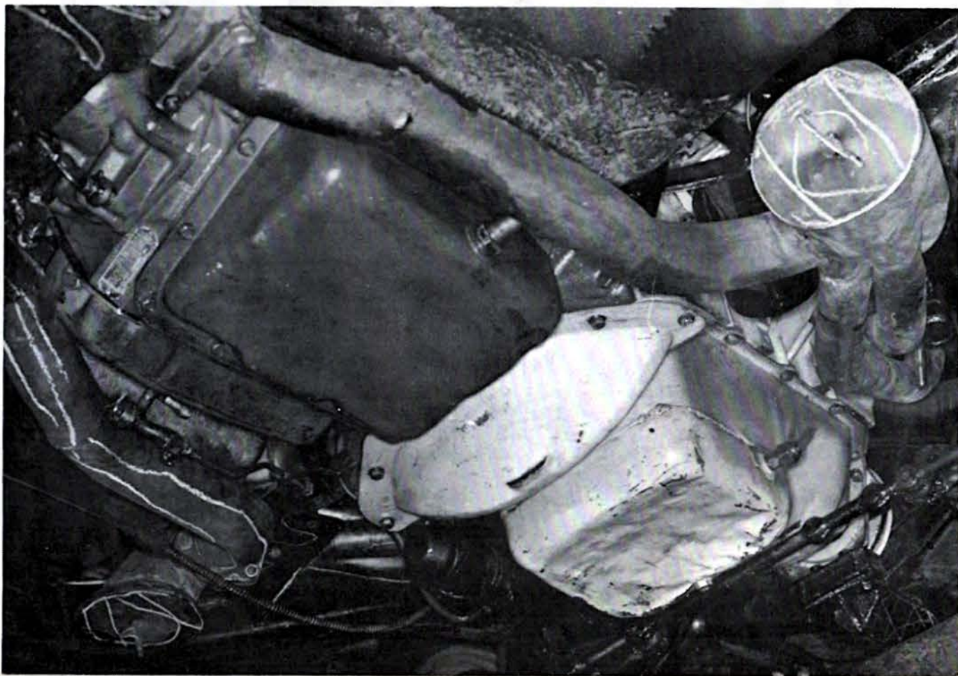
Huge 2½ inch exhaust pipes run from the collectors to the mufflers.
