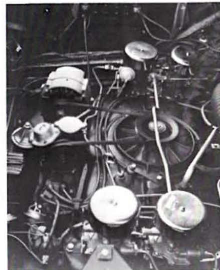
Fitch's Corvair had the stock 4 carb mill with some of his goodies: low restriction mufflers, special air cleaners, bigger carb jets, and reworked ignition system.
