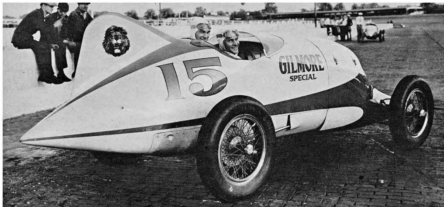
WIND TUNNEL tests aided design of Sparks' "Catfish" for the 1932 Indianapolis 500. Driver Stubby Stubblefield and riding mechanic Otto Wolfer were running in sixth place when a fuel leak forced their retirement on the 175th lap.
