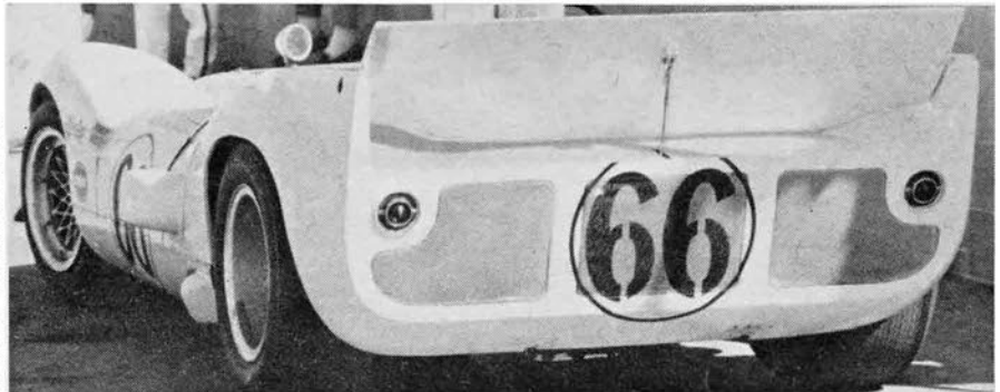
LEFT FOOT operated, a hydraulic cylinder actuates the control rod to tilt the spoiler airfoil and change rear end loading to meet course requirements.
