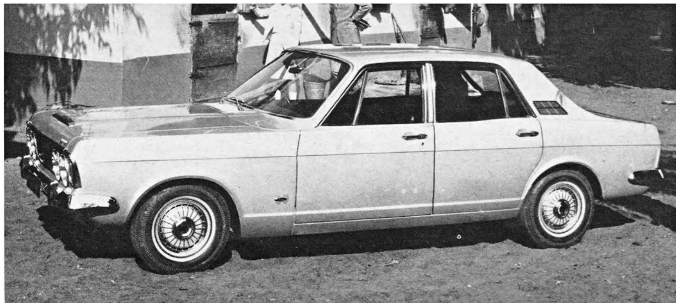
INDEPENDENT REAR suspension, V-6 engines in 152- or 183-cu. in. displacements and an entirely new 4-door sedan body are offered with Ford of Britain's Zephyr/Zodiac twins. And there's a choice of 3-speed automatic or 4-speed manual gearbox.
