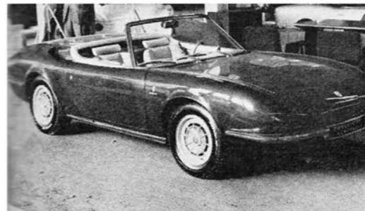
BERTONE-bodied Porsche features slotted headlamp covers which transmit some light when closed.
