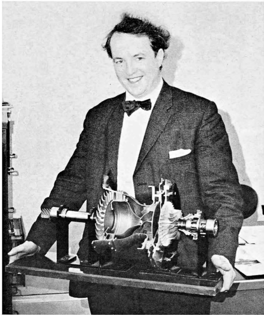
ROVER ENGINEER demonstrates the light weight and compactness of the moving parts in a gas turbine engine. This unit develops 150 bhp.
