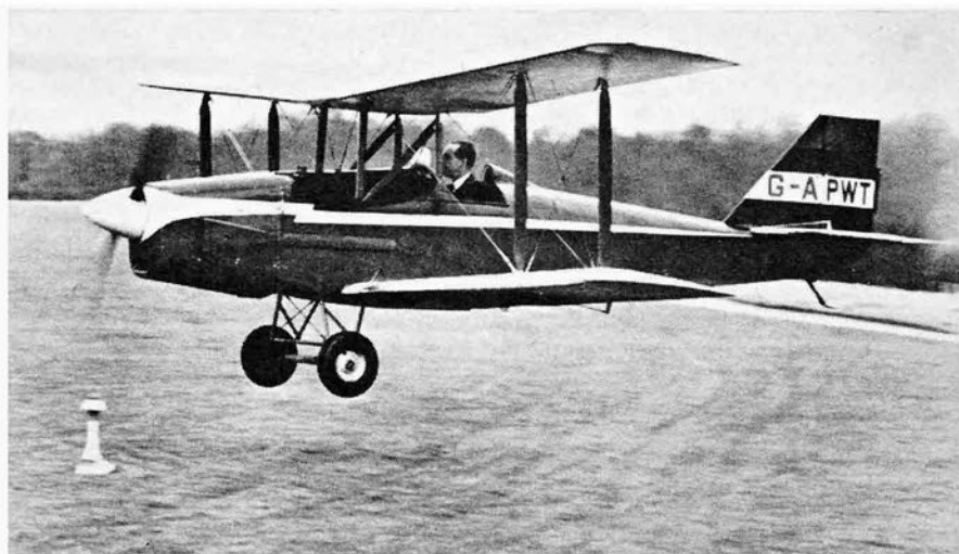
TINY TURBOPROP engine, developing 60 bhp at cruise, was tested in a Currie Wot biplane in 1961 as a by-product of Rover engineering.
