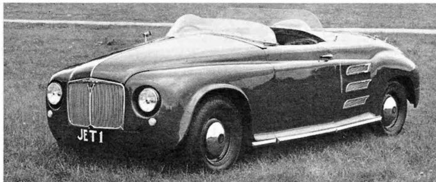
JET 1, the world's first turbine car, was produced by Rover in 1949. The car, timed at 150 mph, now is a museum exhibit.
