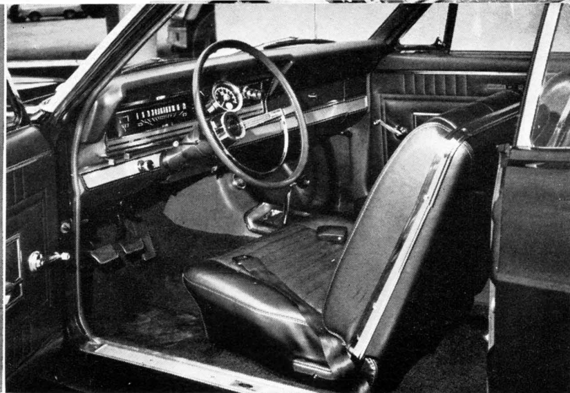
Fairlane's interior is identical to any GT job with the exception of 9-grand tach mounted to right of steering wheel. Though not available yet, C6 Ford-O-Matic is coming.
