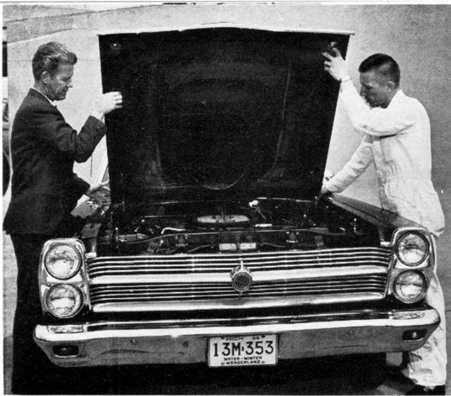
Bill Holbrook, left, and Rolf show filter pack and air cleaner top can be removed to receive direct shot of atmosphere blasting through functional hood scoop.
