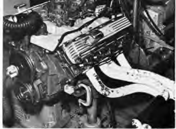
Here you can see 10-inch extensions (no paint) that clamped on an additional 5 horses. Pipes dumped into 11-inch collectors and "clover-leaf" transition pieces.
