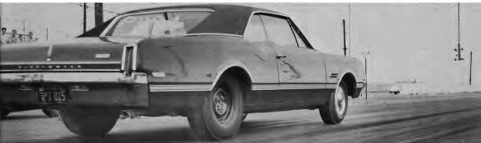
The anti-spin rear-end kept traction on both tires equal. Here car is using a set of slicks for bite.
