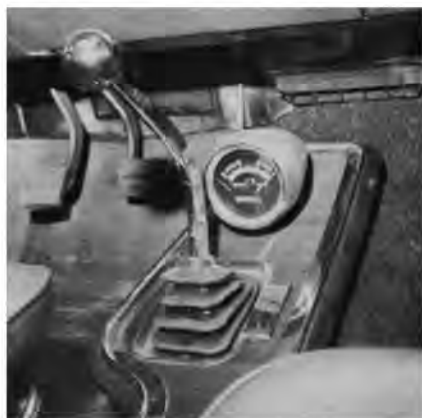
Tachometer location is good as eye distraction from the course is slight. A Hurst shifter is used to handle powershifts or normal shifting techniques.
