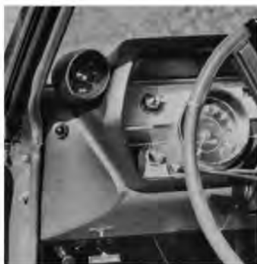
Tachometer location is good as eye distraction from the course is slight. A Hurst shifter is used to handle powershifts or normal shifting techniques.
