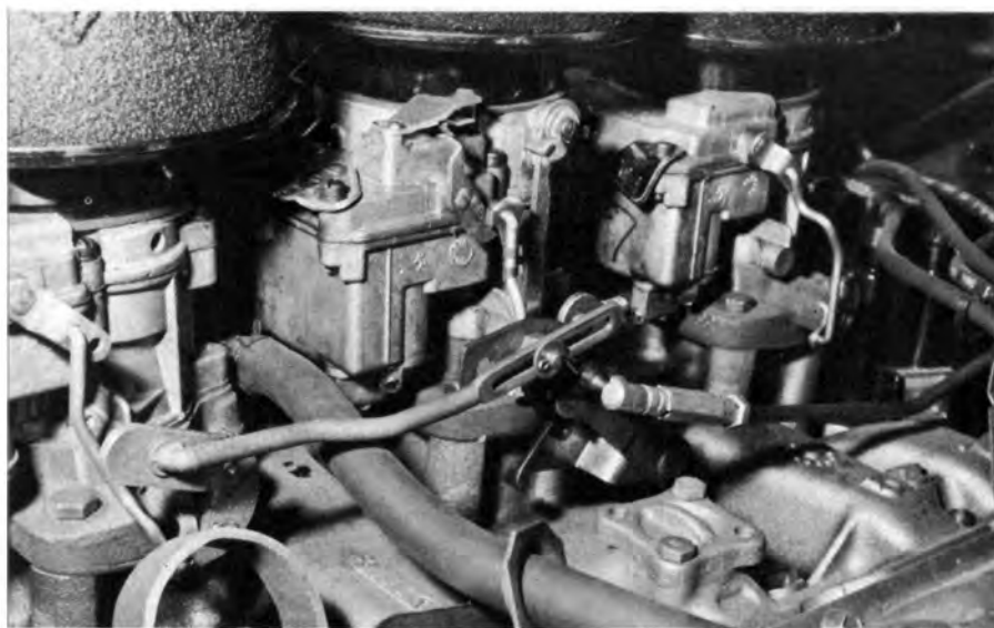
Timing and dwell was checked by Dan Horan, who drives the Allen Paul Oldsmobile 4-4-2. Best timing was slightly advanced from stock setting. Three carbs are of Rochester make and listed as optional equipment.
