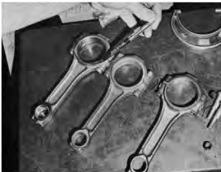
CSC rods are 327 Chevy type. Extensive rework strengthens each unit for performance use. Pin points to reinforcement around crank end.
