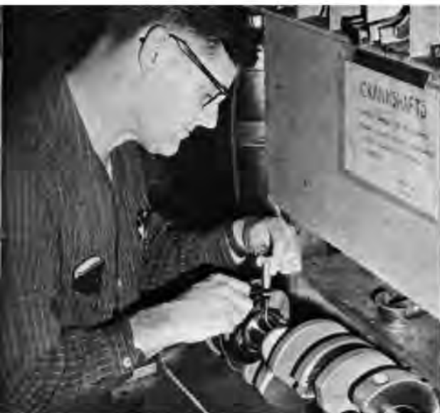
Finished Dyna Rev crank receives final inspection by Alex Alexander, owner of CSC. Straightness, index and throw sizes are double checked. Crank has been magnaflux checked three times.
