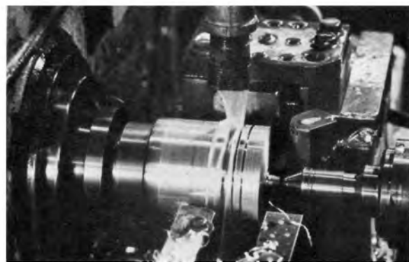
Pistons are rough machined on automatic lathe. Final sizes are cam ground for perfect concentricity.
