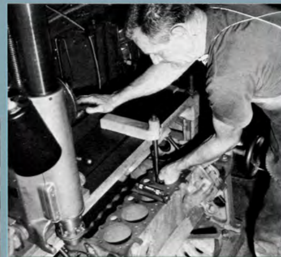
John Ryans trues engine block to Quick Way boring bar. Block mounts at main bearing pads and cylinders are bored at the crank angle. Old boring bars bored at block deck angle.
