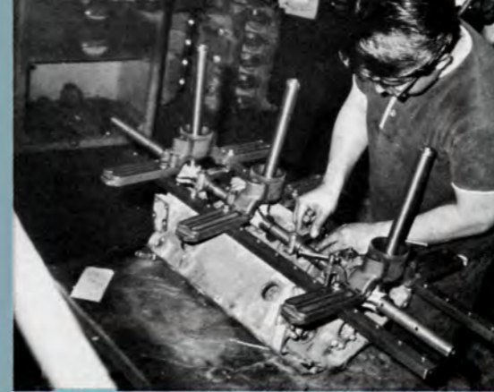
Align boring evens and trues the main bearing mounts. Main caps are removed and milled .018 inch to even caps prior to boring process.
