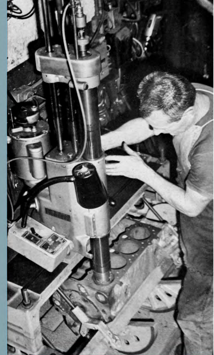
Each main bearing bore is machined individually. The process is very time consuming — but worth it. The engine will gain approximately 500 rpm from the job.
