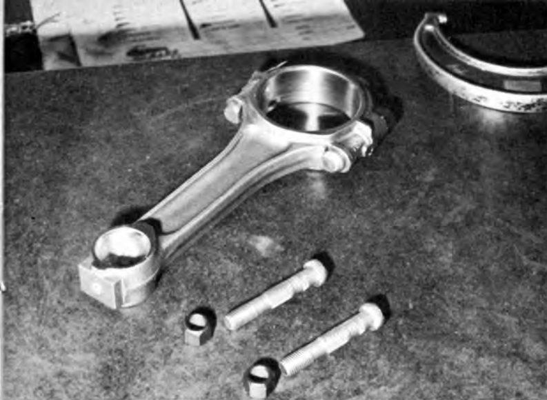
Special high stress bolts replace stock type. CSC has found these to make higher rpm engine speeds safer.
