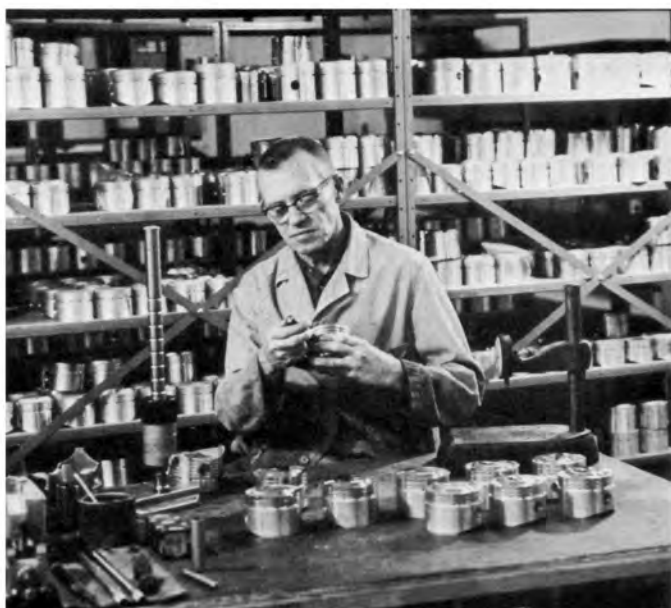
Final inspection of JE pistons includes micrometer inspection of skirts, pin bores and ring land depth.
