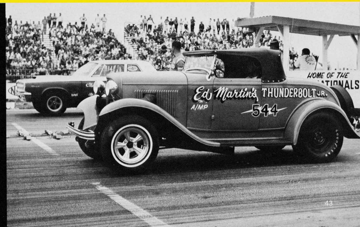
A few big-inch "hot rods" are seen in A/MP. This is a '32 Ford roadster with late 427 Ford high-riser wedge. Wheelbase is 106 inches and weight just over 3000 lbs.
