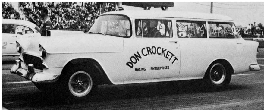
A promising combination for D/MP is the 265-cubic-inch Chevy V-8 engine in '55-'57 Chevy station wagon body. This makes minimum weight of 3450 lbs. easily, and station wagon body gives more than 55 per cent of total weight on rear wheels for maximum off-the-line traction.
