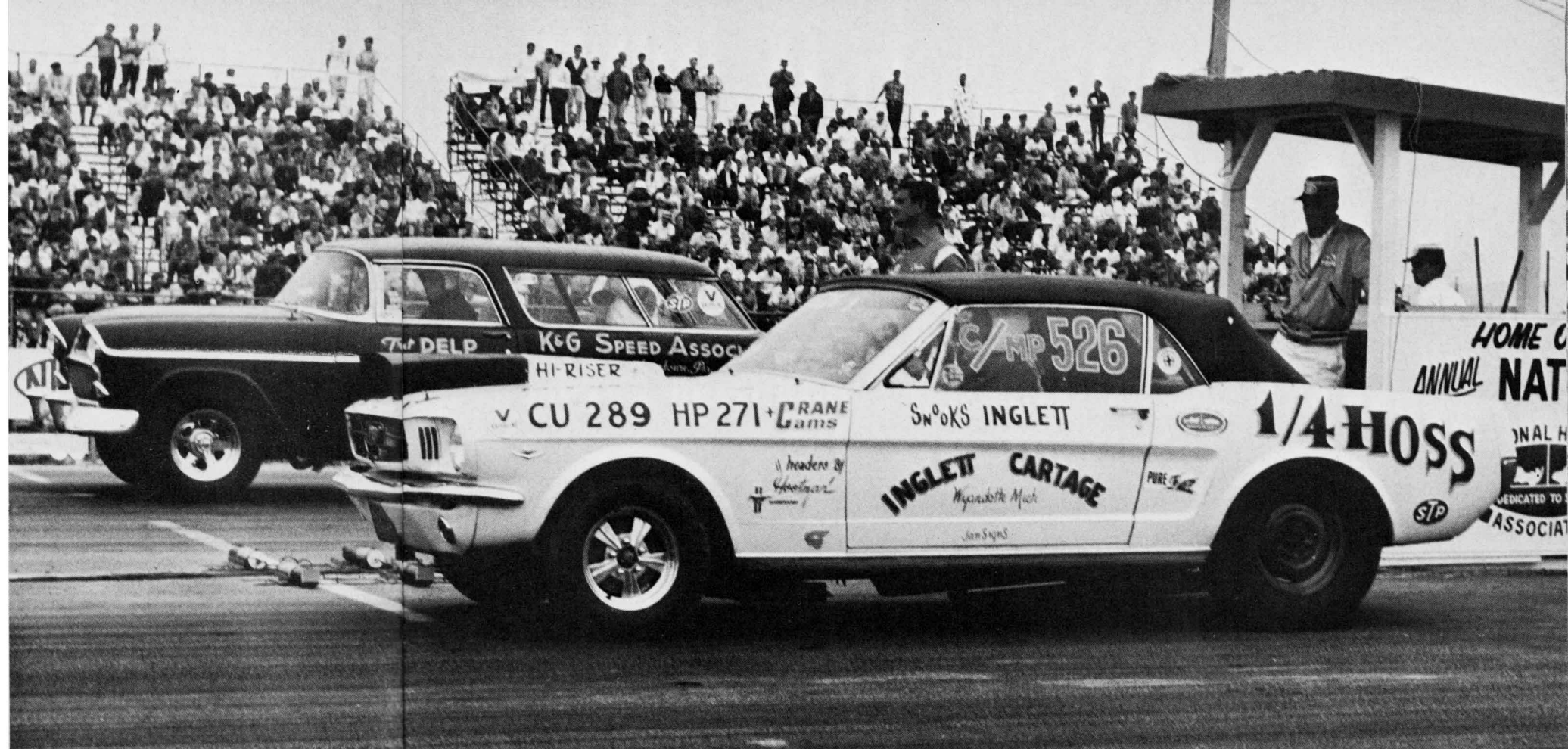
Mustangs with 289 engines are popular in C/MP (minimum 11.00 lbs. per cubic inch). Minimum weight for 289 cubes is 3180 lbs. ET's in the mid-12 seconds at 110 mph are common in this class.
