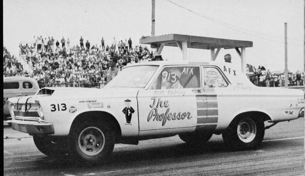
Late Super/Stocks and A/FX jobs like this Plymouth A/FX are seen often in the A/MP class. Car weight with 426 cubic inches can be reduced to 3000 lbs. instead of limited to 3400 lbs. in S/S and 3200 in A/FX.
