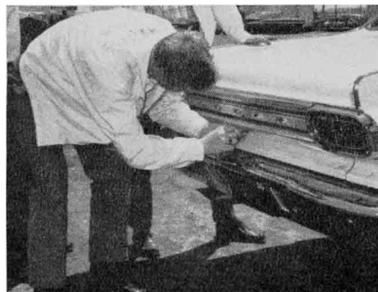
Right — Spare tire is located under trunk floor and lays in flat position. Covering is by means of a piece of fiberboard which is in turn covered with a light rubber mat.
