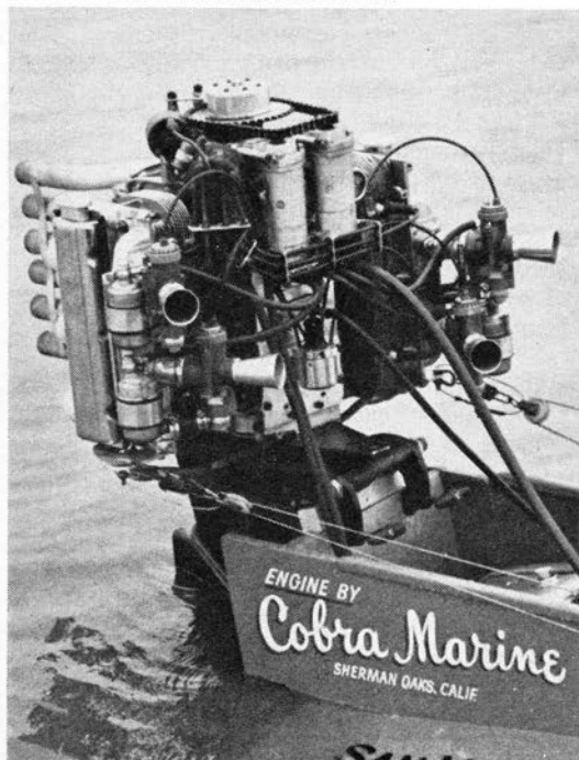
THIS OUTBOARD , magneto sparked and motorcycle carburetored, is a Chevrolet Corvair Six.
