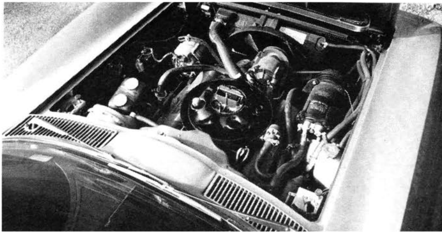
INSTALLATION of standard 327-cu. in. engine leaves enough extra space for air conditioner, emission-control pump and power accessories.
