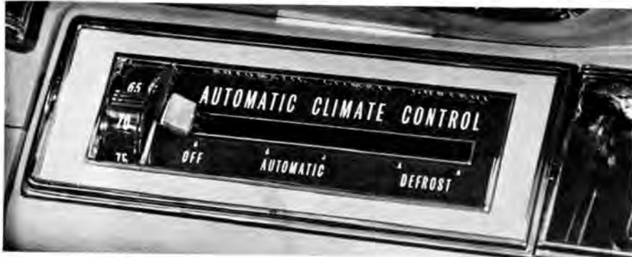
TEMPERATURE SENSOR inside car transmits signals which open vents, valves, switches and ducts that regulate compressor, vacuum system and blower.
