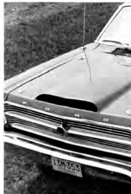
SCOOPED fiberglass hood will be part of an A/Stock Fairlane powered by Ford's 427-cu. in. wedge-head engine.
