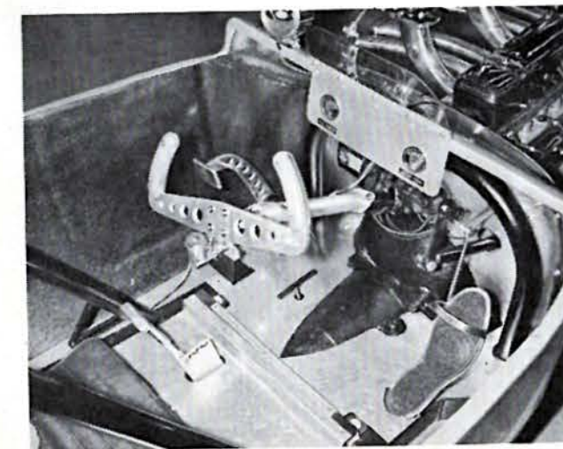
Above, custom ratchet shift handle controls reworked hydramatic. Below, cockpit is uncluttered. Neat airplane-type tiller controls Fiat steering gear setup.
