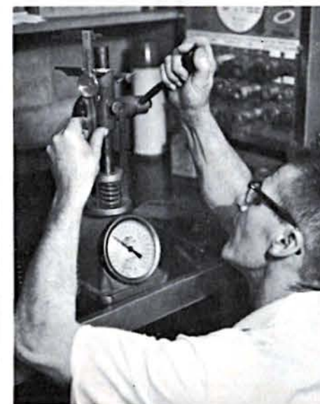
Above, all valve springs are matched for maximum efficiency at 7000-plus rpm. Left, Wally checks every spring for tension at specific seating and opening heights. HP Ford springs are used.
