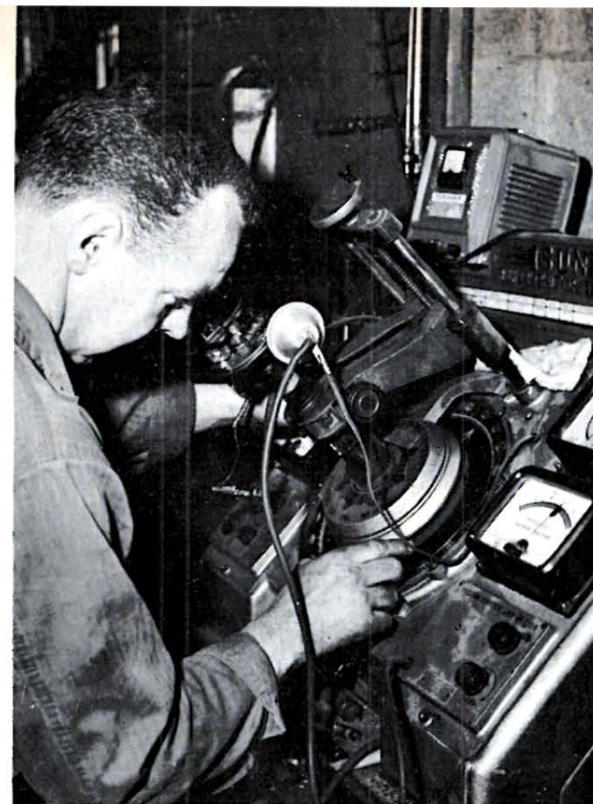
Right, advance curve being built into a Pontiac sparker by Pacers Auto ignition specialist. Below, fuel-burning mill in Gay Pontiac "funny car" sports Crane heads, Hilborn bug catcher.
