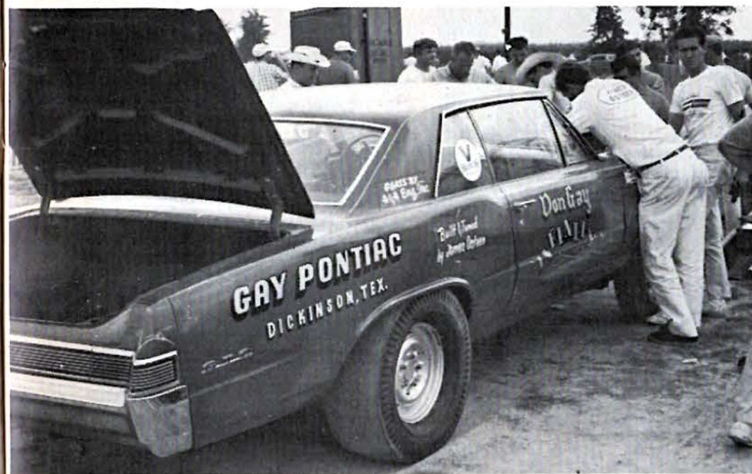
Above, older Pontiac engine is stroked 1/2-inch, bored .060 over for a total of 436 cubs. Left, Don Gay's hottest drag car is this blown injected GTO.
