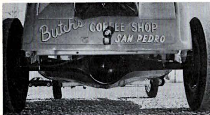
Above, body was channeled six inches. Right, tiller by Covico guides '60 Fiat steering which bolts to a pair of '48 Ford spindles.
