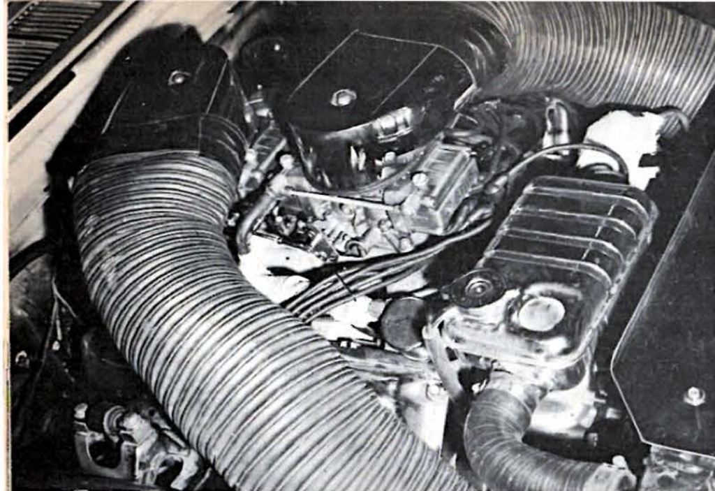
All out dual quad high riser makes use of fresh air "zip tubes" for max breathing.
