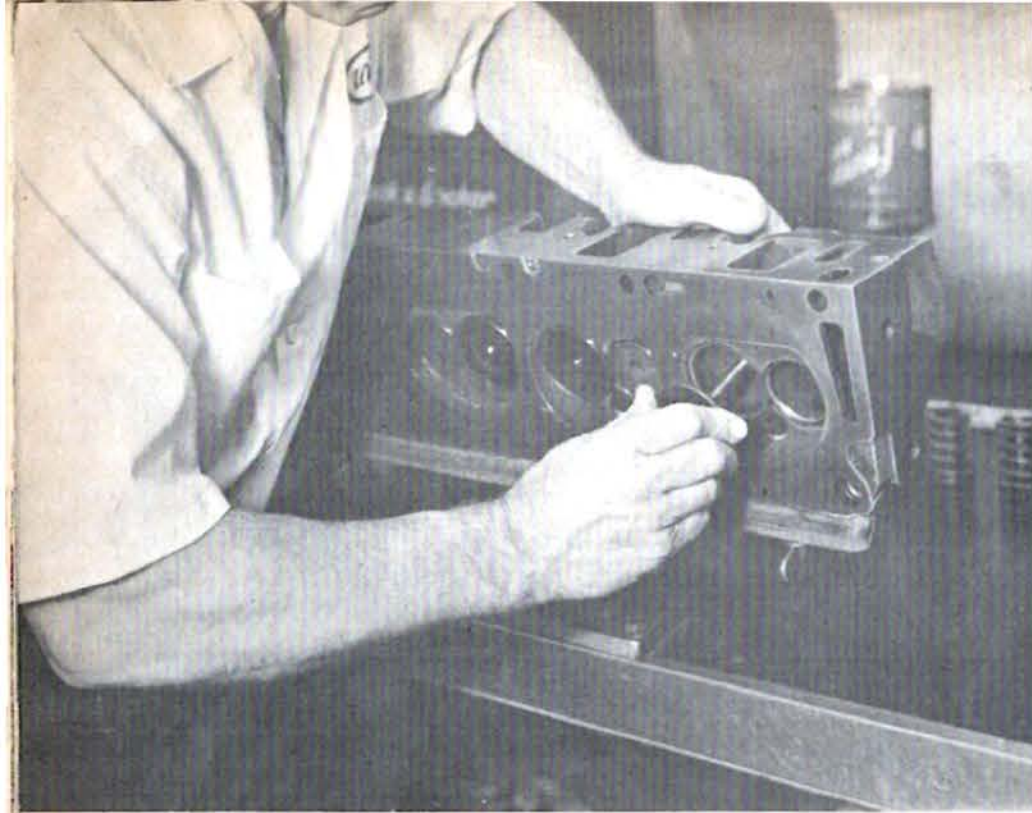
Valves are hand fitted, lapped in for a perfect seat. Nothing is left to chance.
