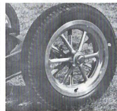
CAE chrome front end supports highly polished magnesium spoke wheels. Bucket seat and integral headrest are padded for maximum comfort.
