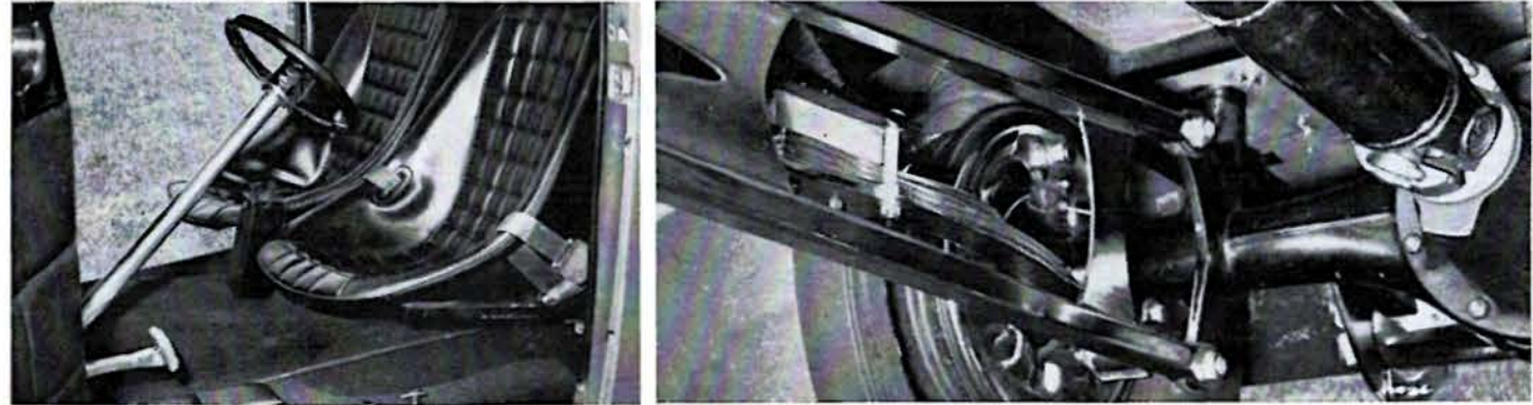
"King Kong's office" was done up in black naugahyde by Style Craft. Steering wheel is a Covico hooked to Volvo unit. Push buttons between seats control trans. Pontiac rear end is suspended with a quarter elliptic spring setup in conjunction with heavy duty shocks. Sturdy traction bars were custom fabricated. Rear end gears are 4.56. All chassis work on car was handled by Ed & Ray.
