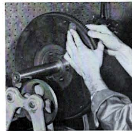
With the mandrel riding on knife-edged rollers, the heavy side of the flywheel goes to the bottom. Clay is added to find light side, then heavy side will be drilled.
