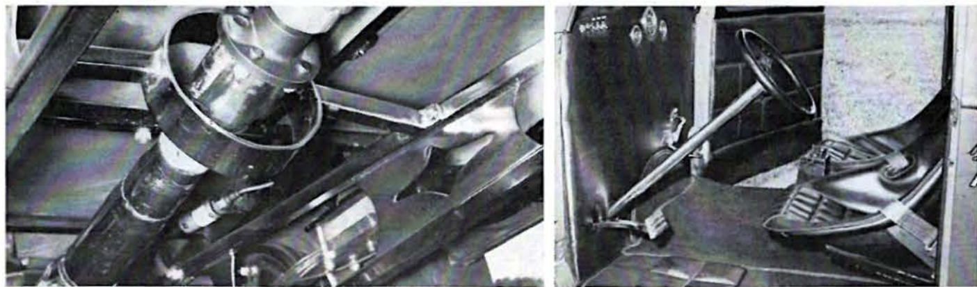
Protecting the driveline assembly should front U-joint break is special frame anchored hoop. Driveline was pirated from a Chevrolet and has not offered any problems. A special adaptor is used at front of drive shaft to mate the unit with modified Torqueflite trans by Art Carr.
