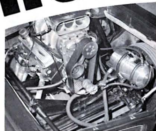
Blown 421 Pontiac features Enderle injectors top side. Blower drive is M/T unit. Inside good stuff includes Crane cam, Forgertrue pistons, stock crank.
