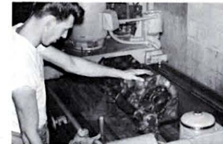
Gary Koehler of Dynamic Engine Service sets up a Chevy block in their Lempco 545BL wet surface grinder. Before mandrel is installed, mains are align bored.
