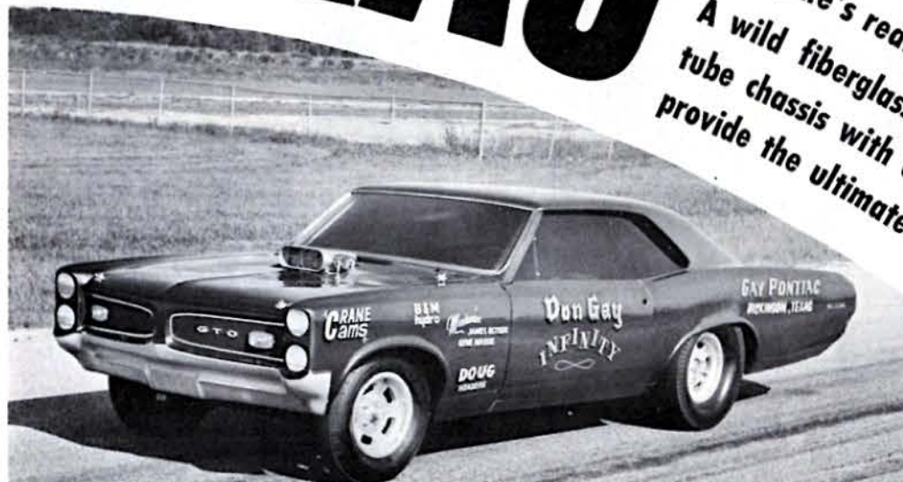
Fiberglass body of GTO was built by A & A Engineering of Atlanta, Ga. Features absolutely stock lines even though front wheels have been moved up seven inches and the rears 14. In first outing in major competition at the NHRA Springnationals, car won class, but lost in eliminator.
