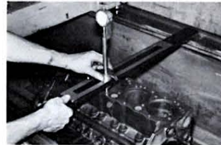
Run of the mill blocks generally require cuts of from .010" to .025" to true them up with the crankshaft axis. This is referred to as parallel grinding or surfacing.
