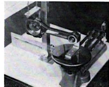
By suspending one end of a connecting rod from a chain or swivel fulcrum, the other end can be weighed. It is important that end weight of rods be held to same figure.
