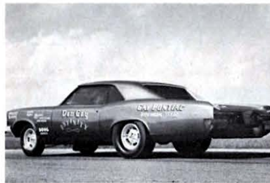
Fiberglass body of GTO was built by A & A Engineering of Atlanta, Ga. Features absolutely stock lines even though front wheels have been moved up seven inches and the rears 14. In first outing in major competition at the NHRA Springnationals, car won class, but lost in eliminator.
