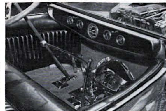
Instruments are by Stewart-Warner, have been set in a wood-grained tunneled fiberglass dash. With carpet removed, chromed trans and bell housing are revealed.
