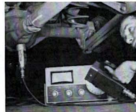
A drive shaft can be balanced directly on the car. An electronic filter system makes it possible to isolate the many driveshaft vibrations from those caused by the axles.
