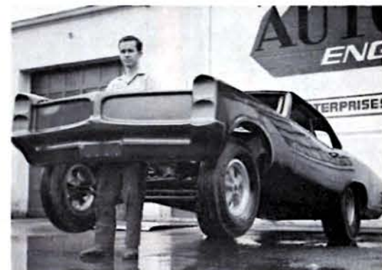
Car builder Jay Howell shows how easy it is to pick up entire front end of car. Minus engine and running gear, machine tips scales just over 410 pounds.
