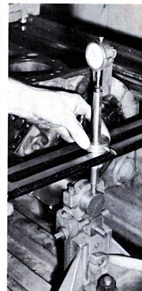
With the true machined mandrel in place of the crankshaft, it is aligned in the grinder by using a dial indicator. The head mating surface is then measured.
