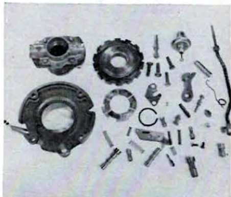
Here are the many components discarded in building the C6 into a racing trans. The large gear at top center is the parking gear, removed if car has a park brake.
