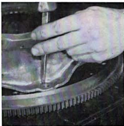
A blunt drift punch is used to stake and tighten clutch cover holes. After clutch and flywheel are balanced, they should be marked to insure future proper alignment.
