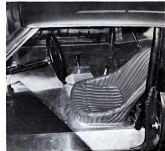
Tube steel frame was constructed so as it would "flex" enough to give good weight transfer. Design incorporates good beam stiffness (up and down bending) but by bowing out the sides, also maintained low twisting stiffness. Main rails are 2" o.d. tube with .060" wall.
