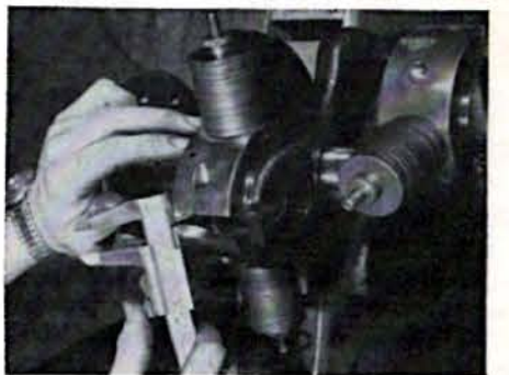
For accurate balancing, even out the gaps between bob weight halves, divide washer weights on rods equally, and center pairs of bob weights on the crankshaft journal.
