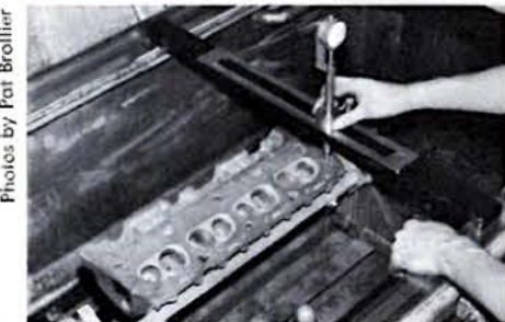
The roll-over fixture is bolted to the exhaust manifold pads and mounted in the wet surface grinder. Dial indicator is then used to check head warpage.
