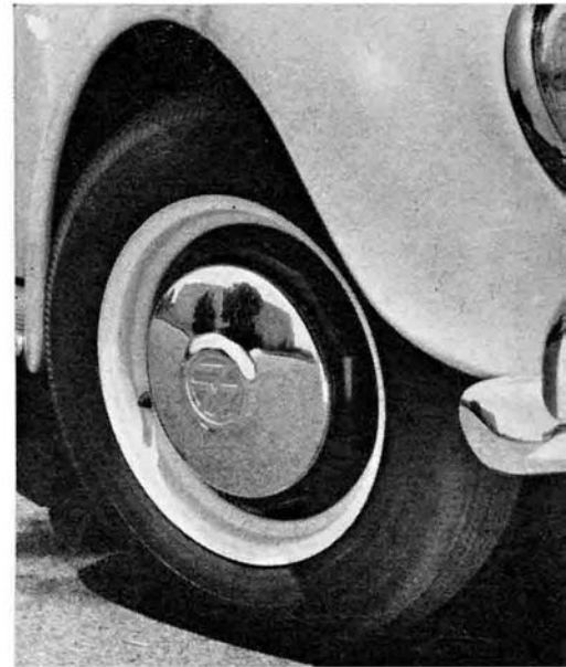
FLATTER hubcaps identify 1300 models. Change was made to reduce curb damage.
