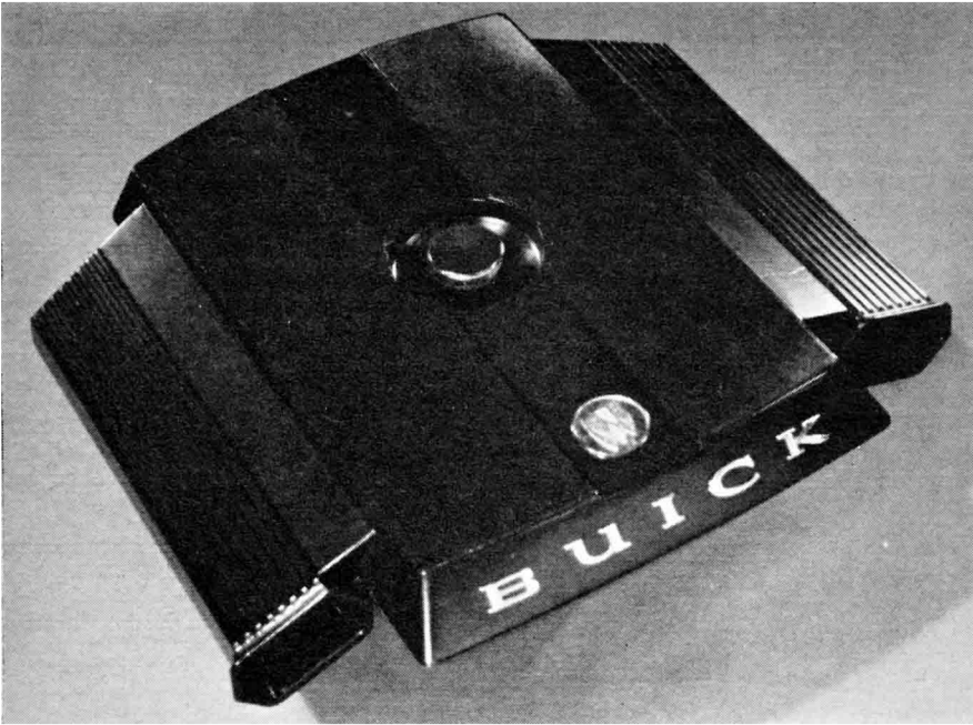
A SINGULAR air cleaner of rectangular shape covers a Rochester Quadrajct carburetor on 400- and 430-cu. in. V-8s from Buick Division.
