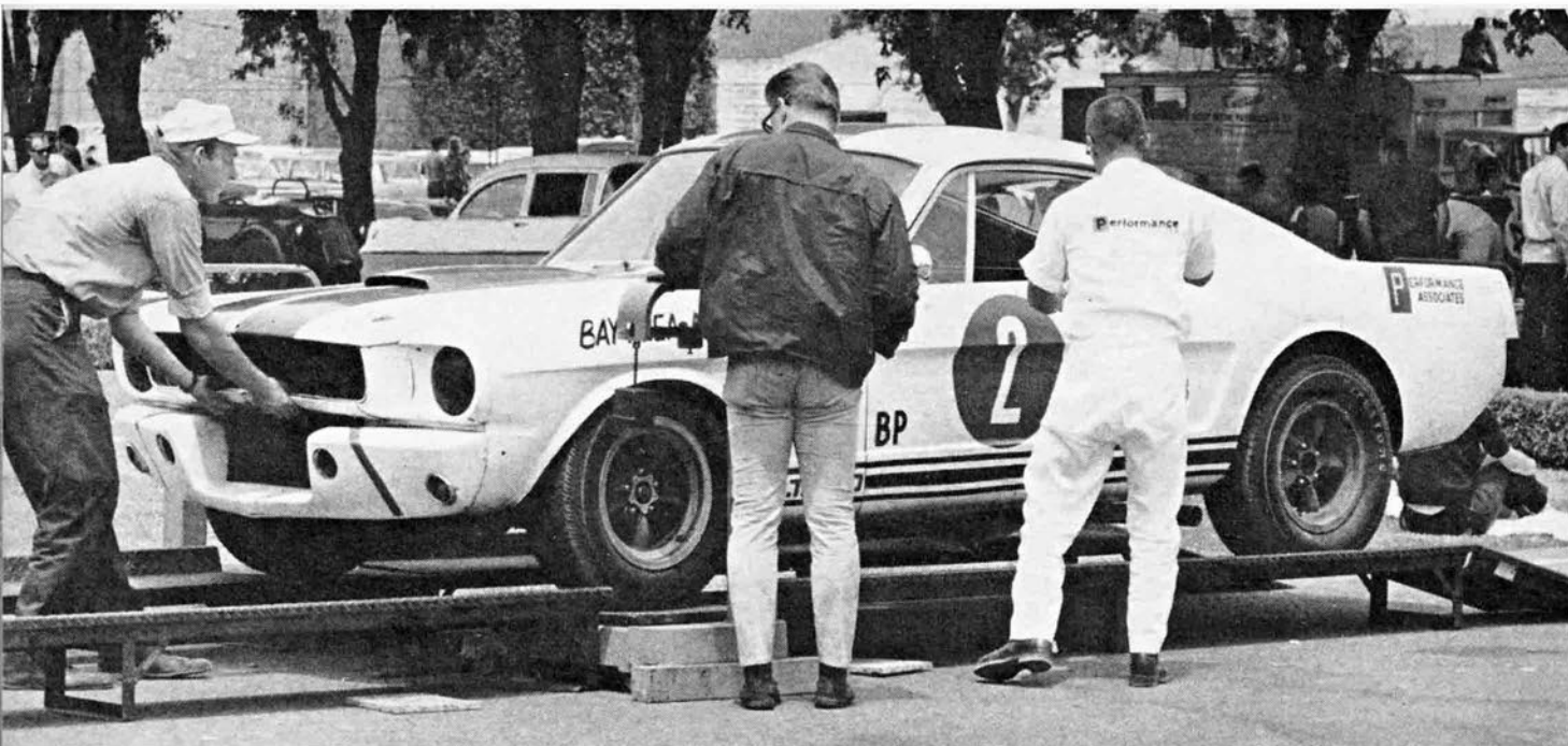
AT RACEWAY weigh-in, a Mustang is checked to determine if it falls within poundage limits. Fastback GT-350, however, doesn't run in sedan classes since it hasn't been homologated with FIA. Appendix J stipulations put Mustang notch-backs and most U.S. compact cars on the grid in Group Two.
