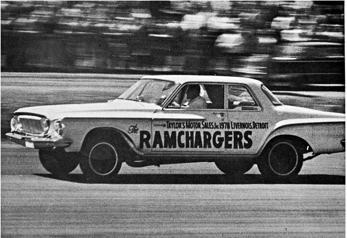
Above, yesterday's Super/Stocks are today's A/S and B/S class cars. This '62 Super/Stock Dodge sports a 413-cube block with special large-port heads and dual quads. It's rated 410 hp at 5400 rpm and has turned 115. Today it runs in A/S class.
