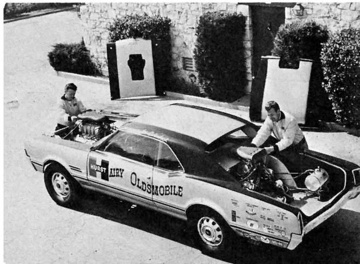
One-off Olds boasts dual blown Rockets, each with its own Toronado drive train. Note stock Toro wheels.
