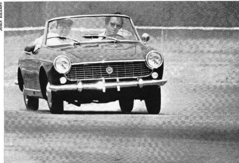
SKID PAD: Establishing steering characteristics.
