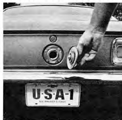
CAMARO has high center-fill fuel tank extension, but no retaining leash on cap.
