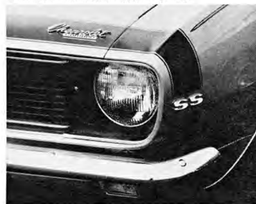
HEADLIGHT option recesses single lamps, covers them with retracting grille panels.
