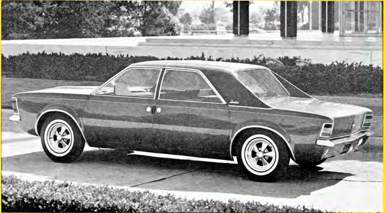
COMPACT CAVALIER offers complete exterior body panel interchangeability which can cut both tooling and consumer costs.
