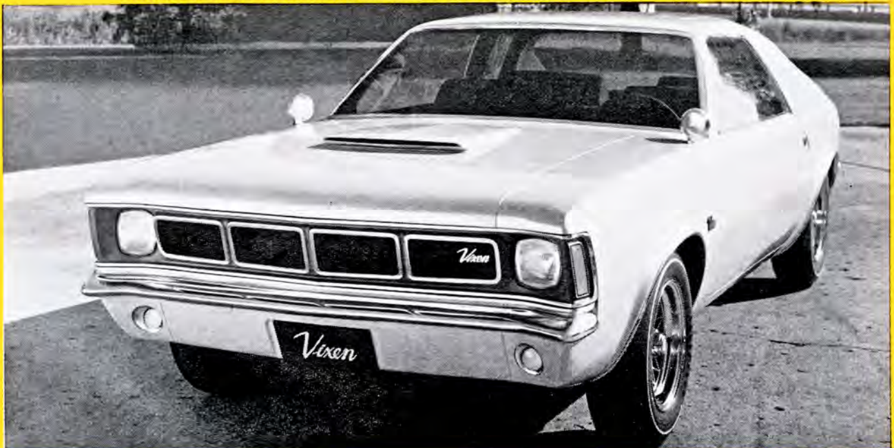
VIVACIOUS VIXEN uses quarter panels identical to Cavalier's, but 1 ft. in length is added at front during stamping process.
