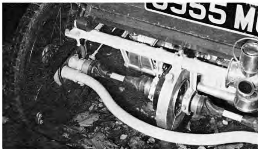
THE ORIGINAL de Dion axle, designed and built in 1900, moved the differential onto the sprung part of the car. I.r.s. isn't new.
