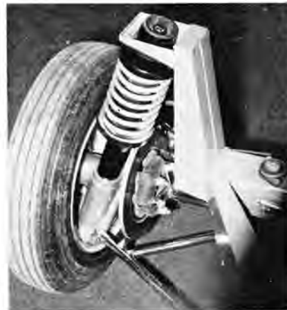
LOTUS Elan strut i.r.s. is related to MacPherson struts used in i.f.s.
