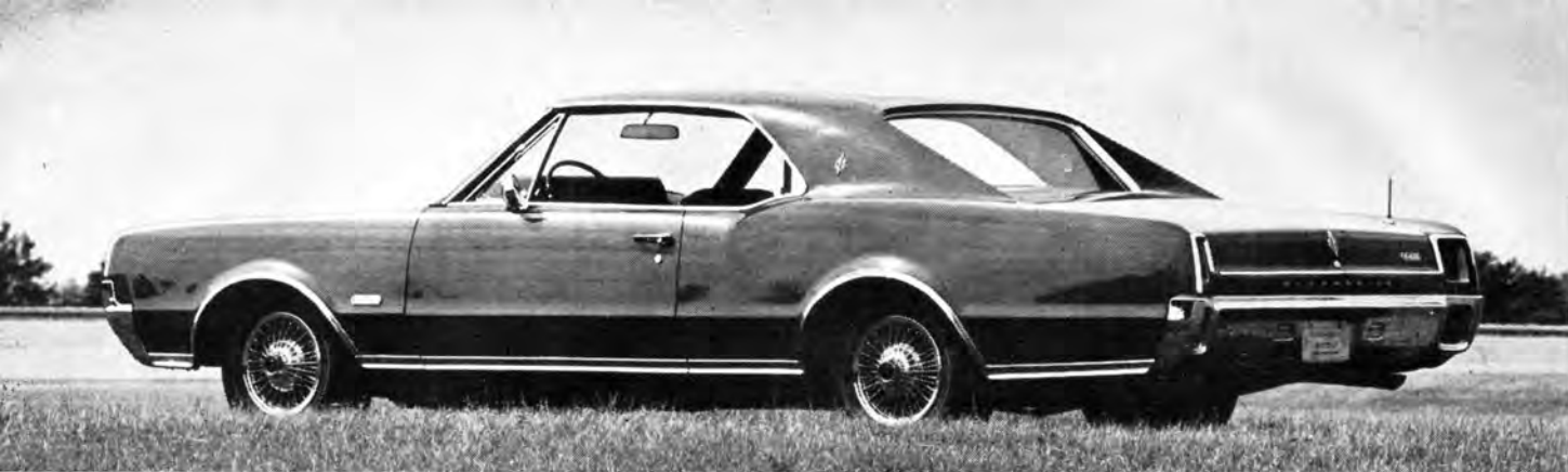
115-IN. WHEELBASE, 204.2-IN. LENGTH AND THE GM "A" BODY'S CHARACTERISTIC FAIRINGS ON REAR WINDOW CARRY OVER FROM '66.
