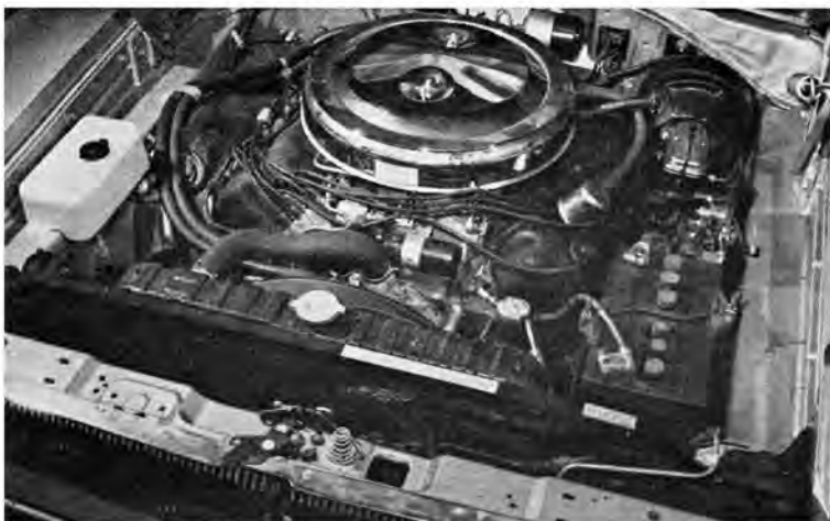
Beefy 425-hp hemi, a $900-plus option, nestles snugly under the Charger hood but with ignition topside, service is easy.
