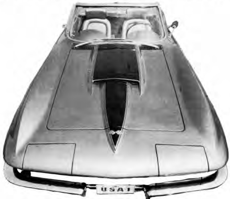
Massive scoop on 427 'Vettes needs only a touch of the coping saw to be functional.
