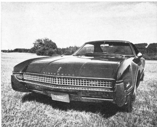
Toronado sits on same 211-in. wheelbase, but disc brakes are a new option. New cam boosts 425-cu.-in. V-8 rating to 425 hp.
