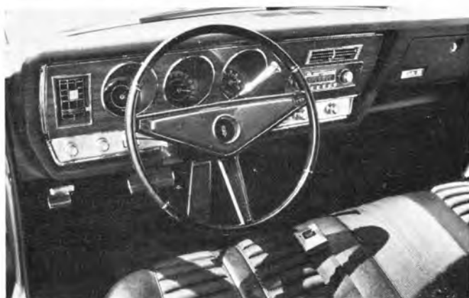
Delta's dash displays new safety consciousness. Nothing protrudes beyond padding, radio is close in, and wheel is padded.
