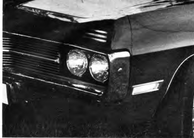
Grille section flips out of the way, exposing headlights. Note eyebrow-hooded parking light, above. Turning lights are options.
