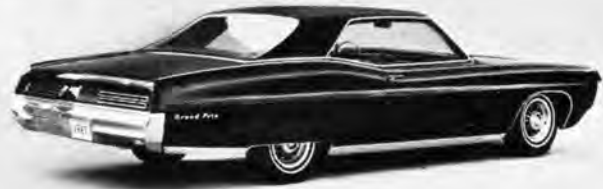
Grand Prix tail light treatment is similar to the GTO, but it has fewer though larger slots. Rear window has concave curve.
