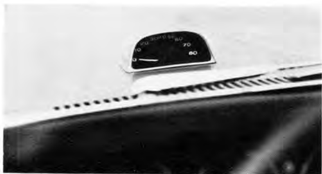
Hood mounting of optional tach permits easy reading, but leaves it highly vulnerable to theft and sheetmetal damage.
