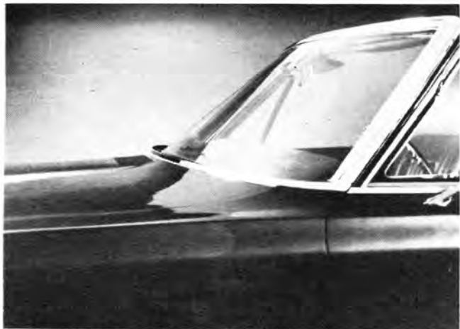
Pontiac people insist there will be no problem of ice locking wipers in the slot. The main advantage is elimination of glare.
