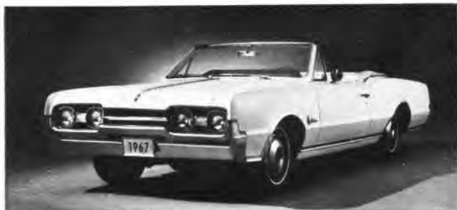
This is the Cutlass Supreme version of the convertible which also comes in 4-4-2 form. Fender extensions are of plastic.
