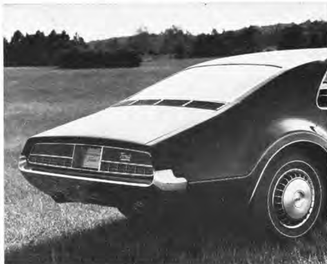
New grille soothes Toronado's blatant tail lights. Vents under rear window are air exit for flow-through ventilation system.
