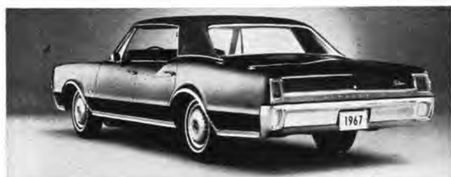
Most popular family sedan will probably be turnpike-cruising Cutlass with 400-cu.-in. 2V V-8. It'll turn 100 mph at 3100 rpm.
