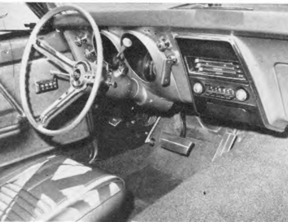
Recessed hooded instruments with conical plastic lenses resemble those of Corvair. The spoke horn buttons are optional.
