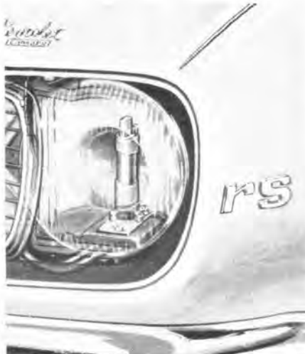
Doors swing inboard to expose concealed headlamps. RS letters denote Rally Sport package which includes concealed lamps.
