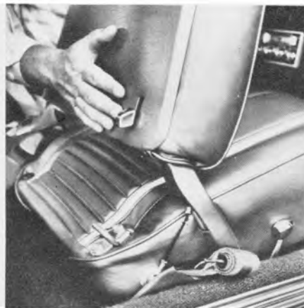
Sturdy-looking seatback latch tends to keep rear occupants from flying forward under sudden impact or severe braking.
