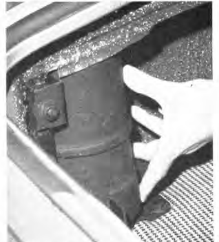
Mysterious looking cannister reposing in left trunk corner of convertibles turns out to be mass damper, tunes out vibrations.
