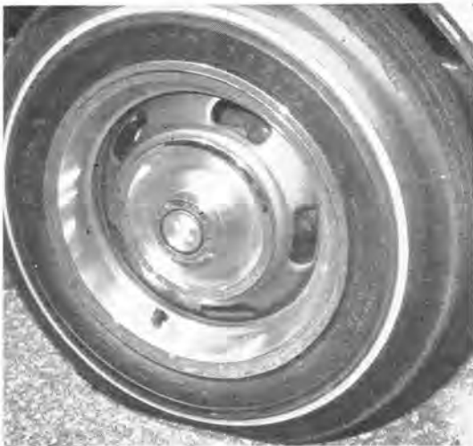
Perforated steel wheels with brushed aluminum beauty rings are all yours when optional Moraine front discs are ordered.
