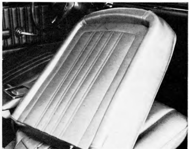
Cougar's seatbacks have energy-absorbing padding for protection of rear seat passengers. Hex screw is for rake adjustment.
