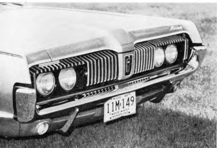
Dual headlamps remain stationary while doors hinge upward and inward, adjustment and aiming remaining undisturbed.
