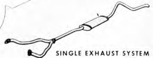
Quiet system for Mustang exhausts maintains engine noise at a non-irritating level.
