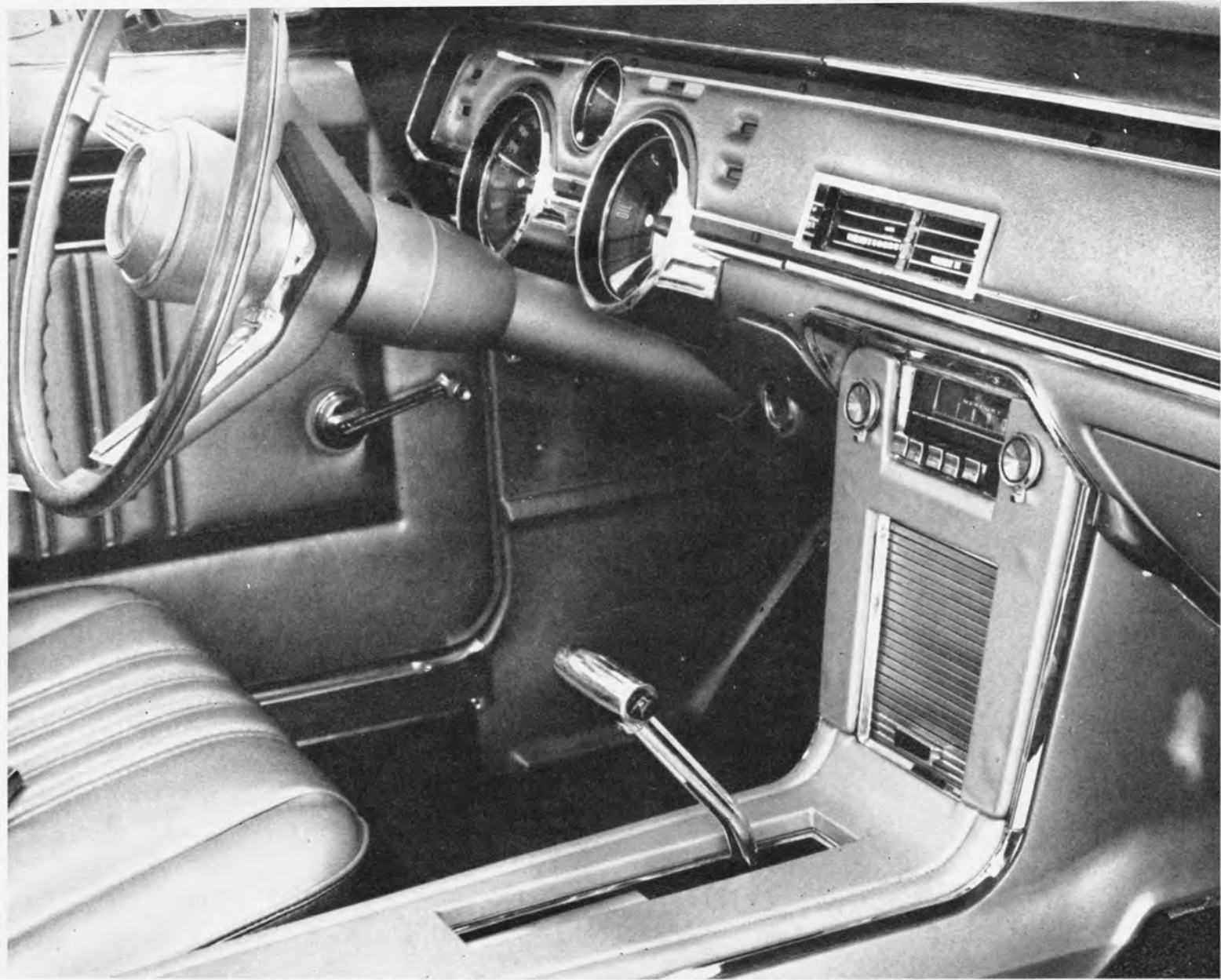
ENERGY-ABSORBING PADDED STEERING WHEEL HUB IS CALLED A "DAGMAR." T-BIRD-LIKE CENTRAL CONSOLE IS OPTIONAL AT EXTRA COST.
