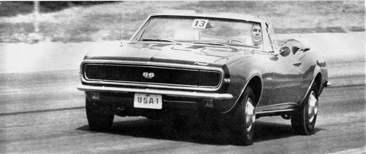
STANDARD SUSPENDED SS 350 LEANS ONLY MODERATELY THROUGH 110-MPH SWEEPER. WIND BUFFETING'S SURPRISINGLY MILD AT THIS CLIP.
