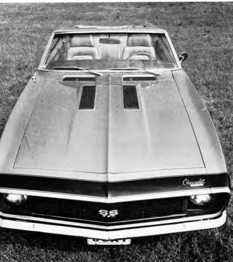
"Bumble-bee" stripes, longitudinal hood louvers mark SS 350 as top-optioned Camaro. Single headlamps have concealing option but are shown uncovered in this photograph.
