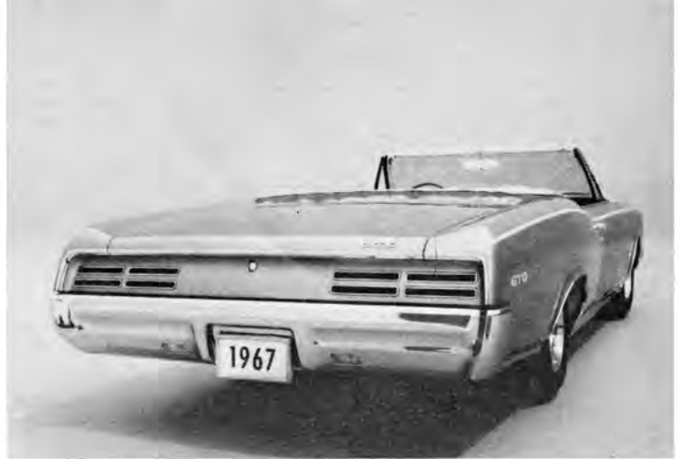
TAIL AND stop lights for the GTO are formed as vents in banks of two at either side.
