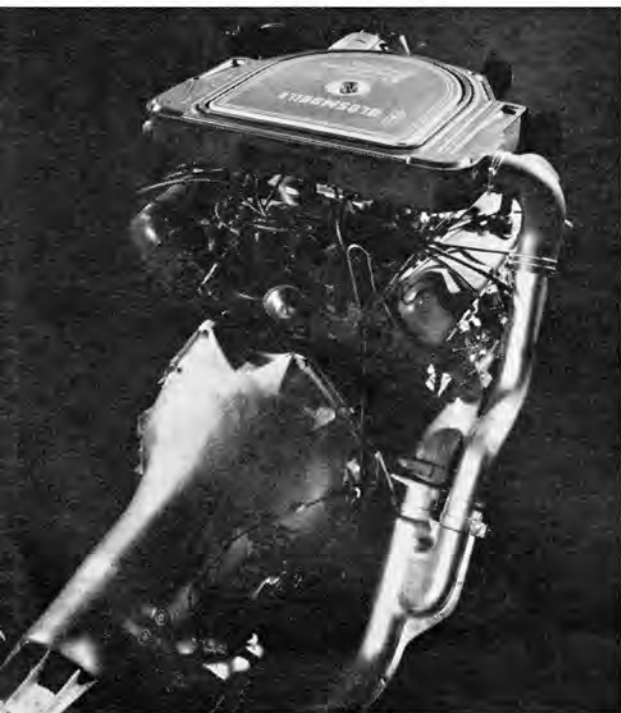
PRE-HEAT air intake system for Olds V-8s eliminates carburetor icing.
