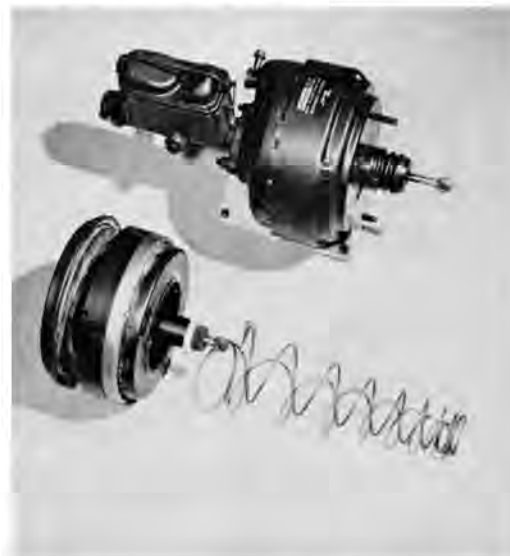
TANDEM VACUUM booster is used by Olds; Buick increased the size of its booster.
