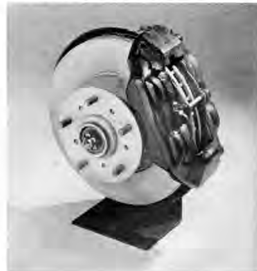
FRONT WHEEL brake discs are vented design with 4-piston calipers.
