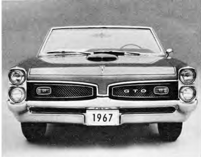
RETRIMMED FRONT of Pontiac's GTO announces an engine of 400 cu. in., an enlargement of the earlier 389.
