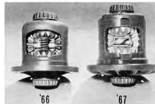
OLD AND new friction discs from Olds' differentials show one area of improvement.
