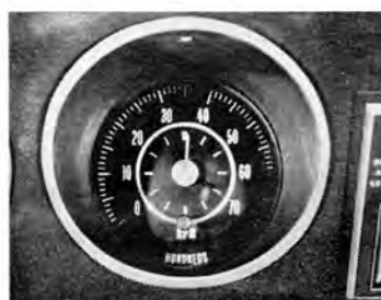
TIC-TOC-Tach , combining clock with tachometer, is Oldsmobile's method of dealing with instruments.
