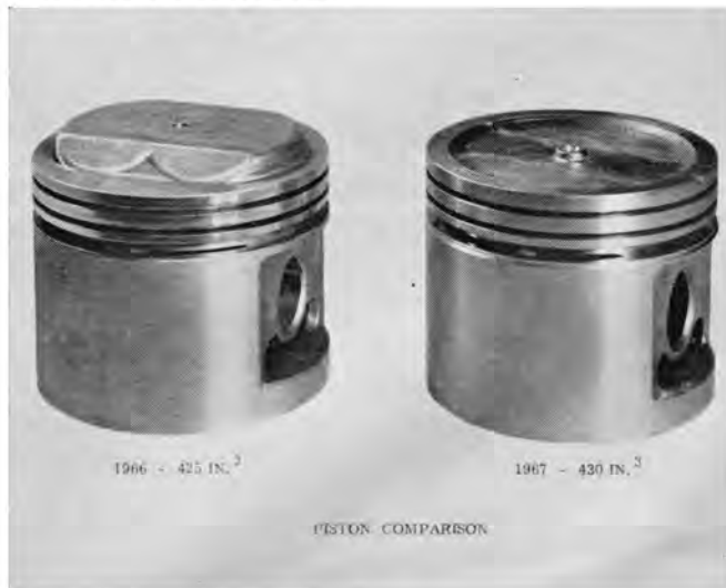
DOMED PISTON crown from earlier pent-roof engine contrasts with the scooped-out crown of the new.
