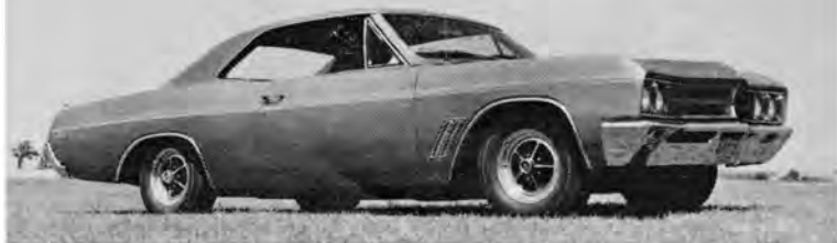
WIDE OVAL tires on special steel wheels place extra rubber on the road to improve GS 400's handling qualities. Louvered vents in front quarter are simulated.
