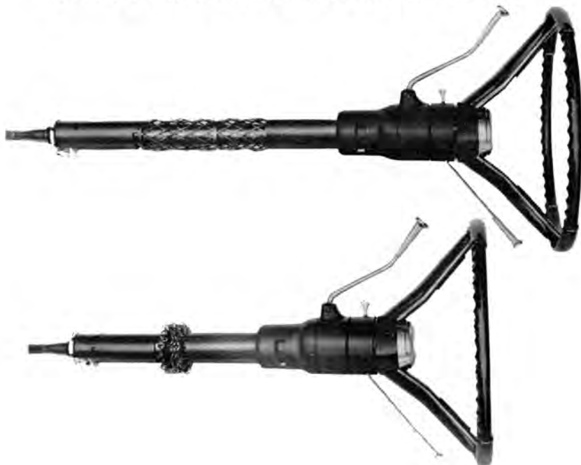
COLLAPSING STEERING column used on all GM cars for 1967 is designed to telescope upon impact. Small knob under shift lever is flasher light switch.
