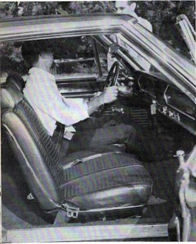
Plush interior is stamped tuck and roll design vinyl with full carpeting. Safety features include lap belts, front and rear, adjustable head rests, yielding rear view mirror and improved sun visor location. Ample leg room is a plus. 40 CAR CRAFT NOVEMBER 1966
