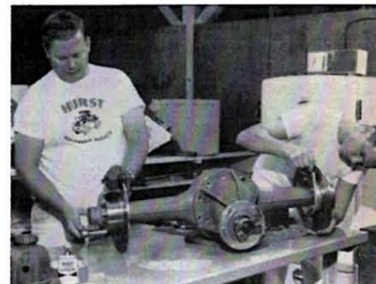
Below right, The aluminum "hat" shown supporting the Airheart caliper bracket also retains the axle/bearing assembly in the housing. It slips over axle first, is followed by bearing, washer, and retaining nut. The "hat" is then bolted to the housing.
