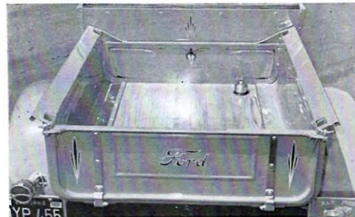
Detailing is clearly evident in the pickup bed with its varnished wooden flooring and perfect side panels. Bed has been shortened 10 1/2" providing a modern appearance. Neat striping is by Averill of Fresno, Calif.
