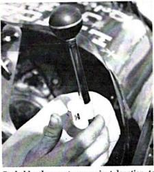
Probably the most convenient location to install a Hurst Line/Loc holding button in a dragster would be on the brake handle. Once the brake is locked, pressure can be released on the handle itself but button must be held down until ready.
