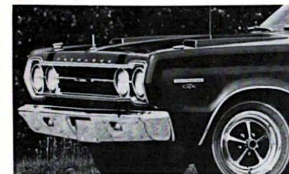
Four horizontal headlights mounted in blackened grille, twin hood scoops highlighted by bold striping, GTX name plates and a racing type pop-open gas cap "give away" Plymouth's new entry in the performance field.
