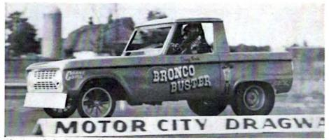
Blasting off the line, Nash's Bronco gets a handful of traction early due to automatic trans. American magnesium spoke wheels give the "Bronco Buster" a real early American look. Slight forward rake to body and bumper angle are conducive to high speed handling.
